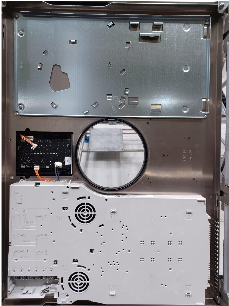
Internal view generator, touch control without blower
