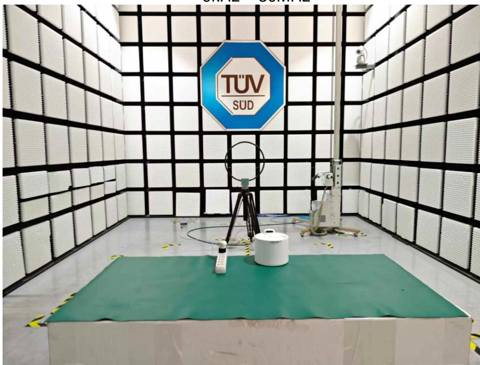
Radiated Emission Setup 9kHz ~ 30MHz
