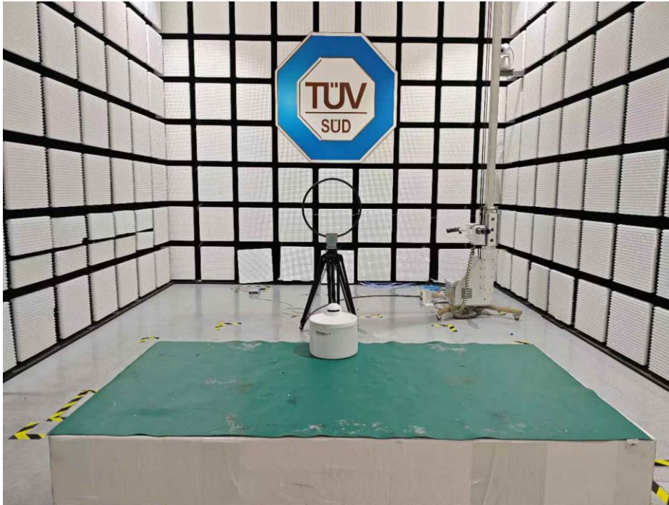
Radiated Emission Setup 9kHz ~ 30MHz
