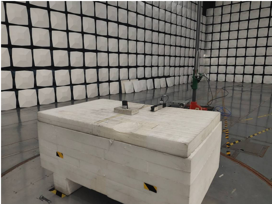
Radiated Emission 9k-30MHz Perpendicular View-Configuration 1#
