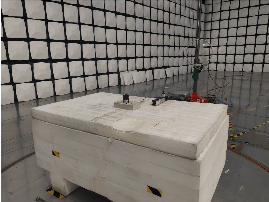
Radiated Emission 9k-30MHz Perpendicular View-Configuration 1#
