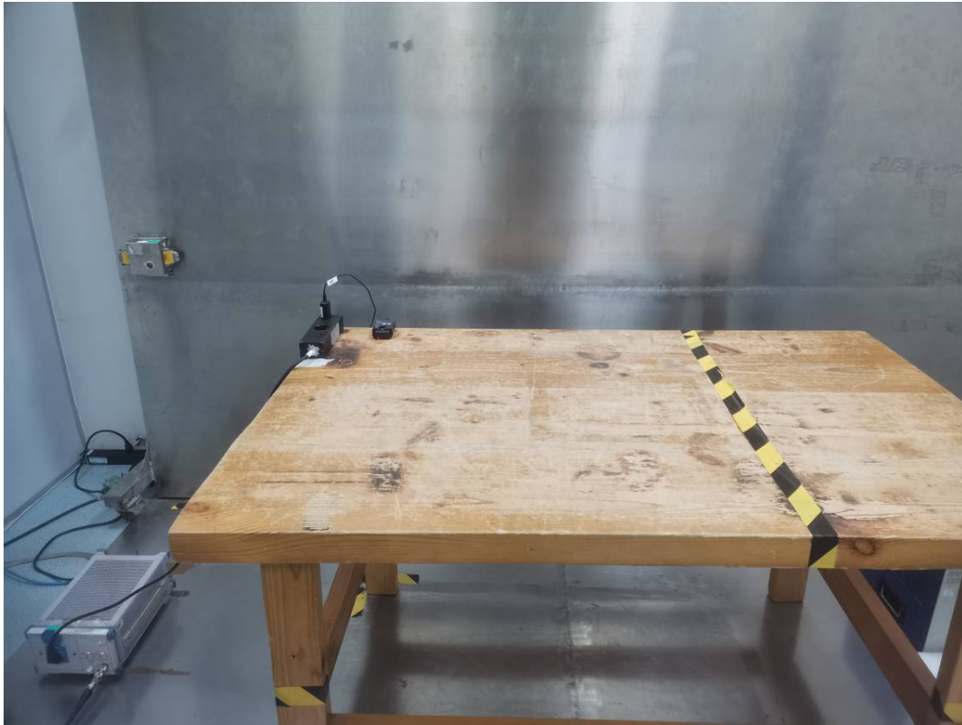
Conducted Emissions Side View-Configuration 2#
