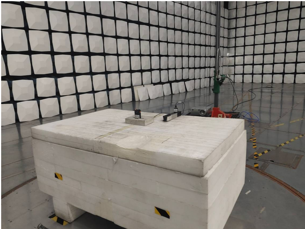
Radiated Emission 9k-30MHz Perpendicular View-Configuration 2#
