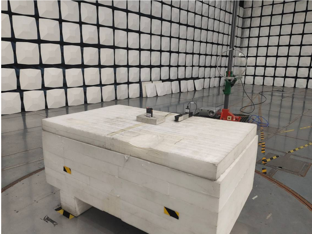
Radiated Emission 9k-30MHz Perpendicular View-Configuration 2#
