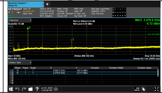
30.0 MHz - 25000.0 MHz \pi/4 DQPSK_2-DH5_Channel 78
