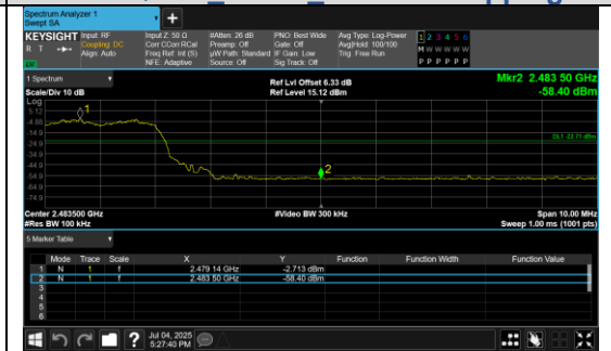
Out Of Band Emission(Right) \pi/4 DQPSK_2-DH5_Channel Hopping
