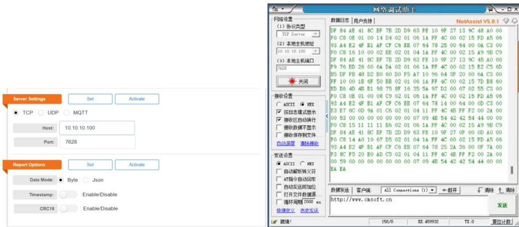
(9) If you need to use MQTT, build your own MQTT server and fill in the corresponding MQTT node address and related subscription topics, as shown in the following figure:
