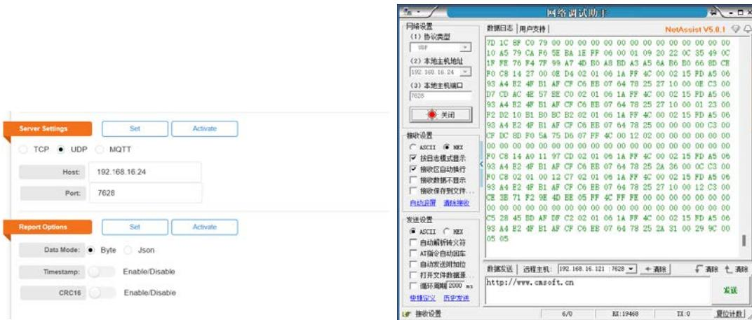
(7) After successful configuration, Net Assist will receive data from the gateway. Can be parsed based on Bluetooth gateway data protocol;
