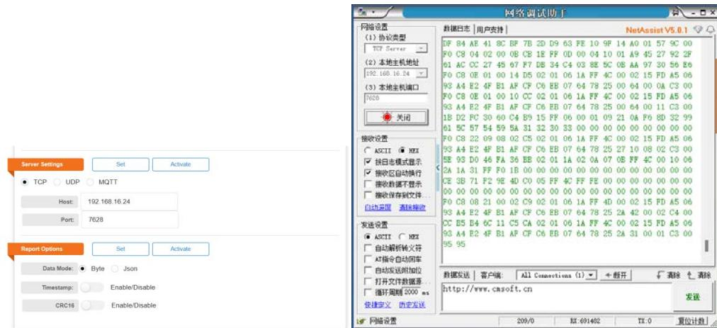
(9) If you need to use MQTT, build your own MQTT server and fill in the corresponding MQTT node address and related subscription topics, as shown in the following figure:
