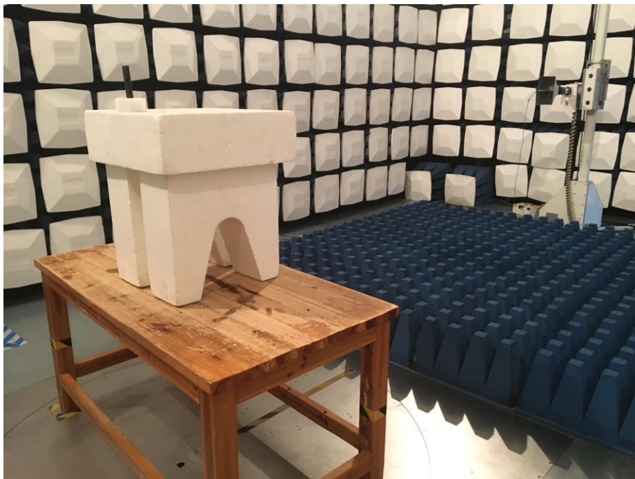
Test Setup For Radiated Emission (Above 1GHz)
