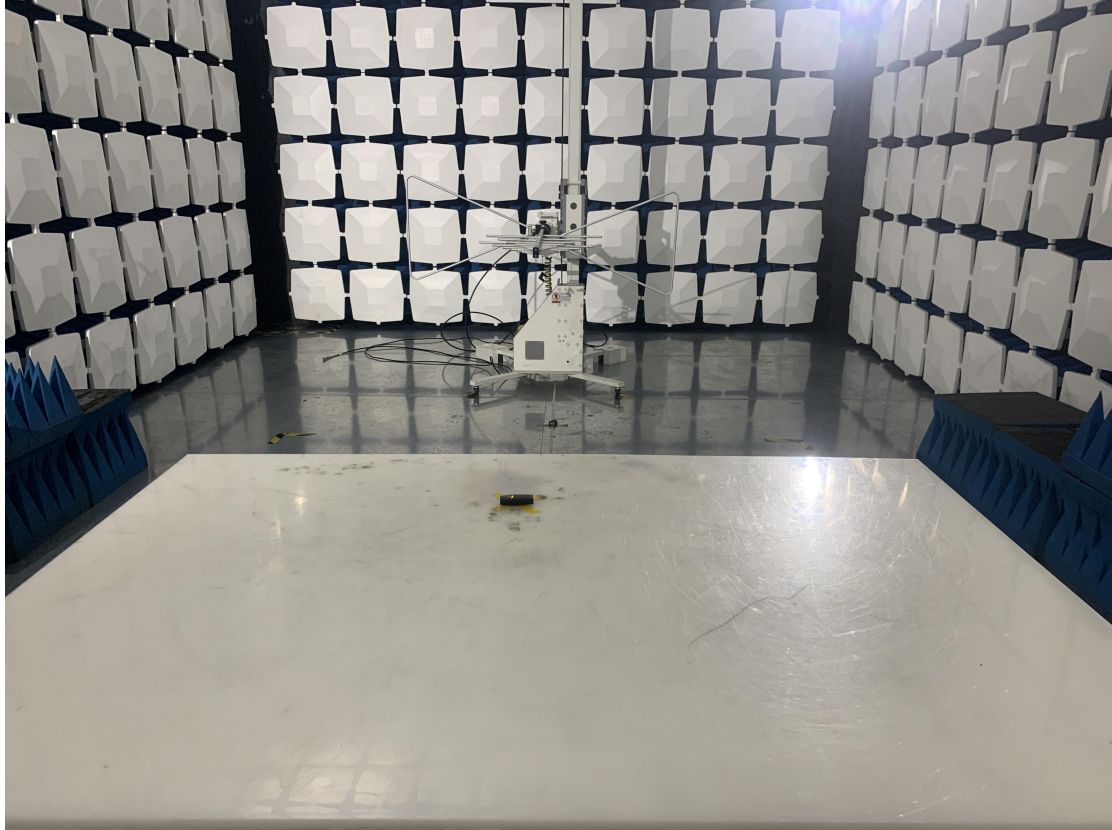
Blow 1GHz for radiated emission test setup
