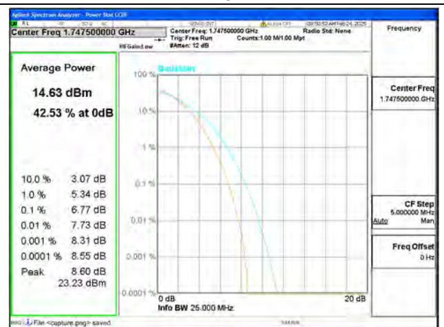
B4 / 15MHz / High CH / 256QAM
