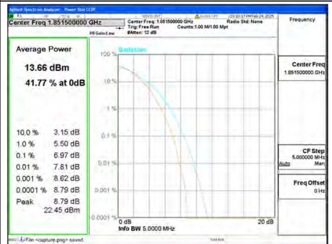
B25 / 3MHz / Low CH / 256QAM
