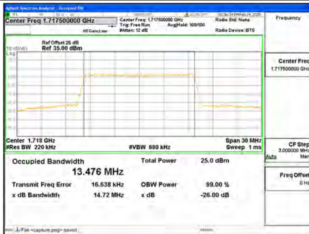
B66 / 15MHz / 64QAM/ Low CH
