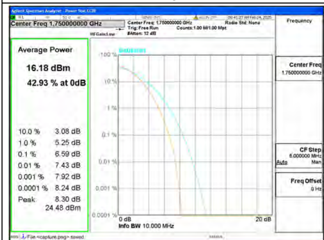
B4 / 10MHz / High CH / 64QAM
