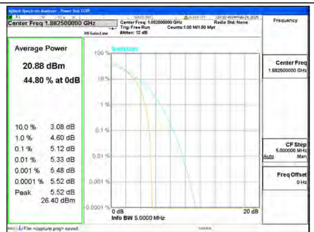
B25 / 3MHz / Mid CH / 256QAM
