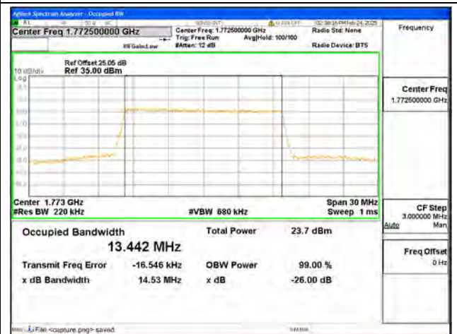
B66 / 15MHz / 256QAM/ High CH
