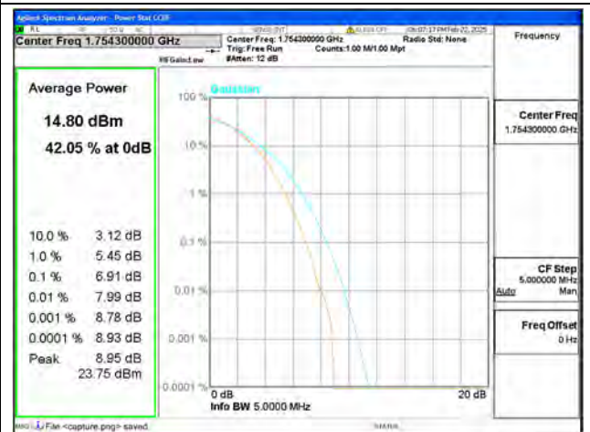
B4 / 1.4MHz / High CH / 256QAM
