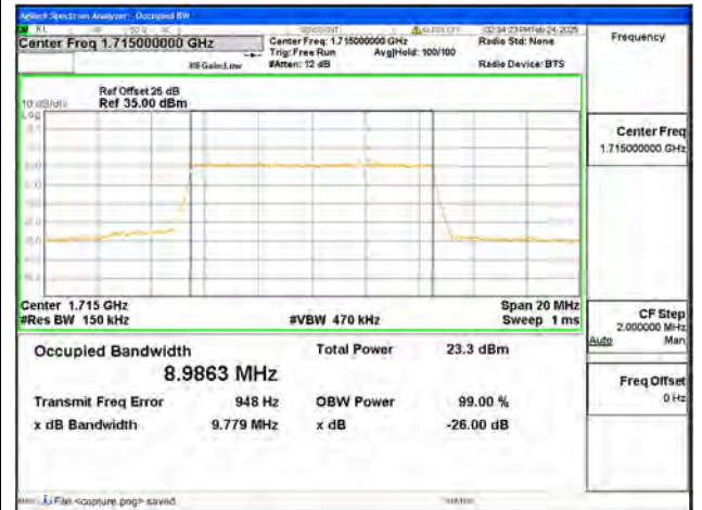
B66 / 10MHz / 256QAM/ Low CH
