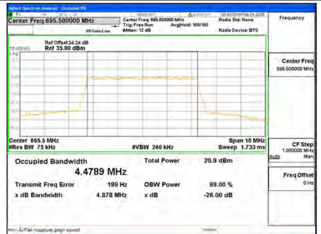
B71 / 5MHz / 16QAM/ High CH
