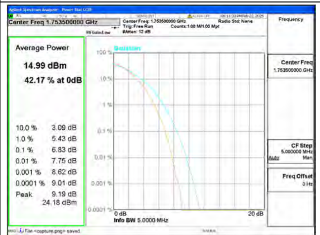
B4 / 3MHz / High CH / 256QAM
