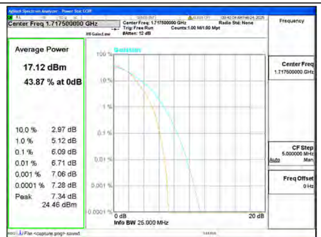
B4 / 15MHz / Low CH / 16QAM
