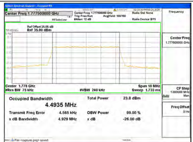
B66 / 5MHz / 256QAM/ High CH
