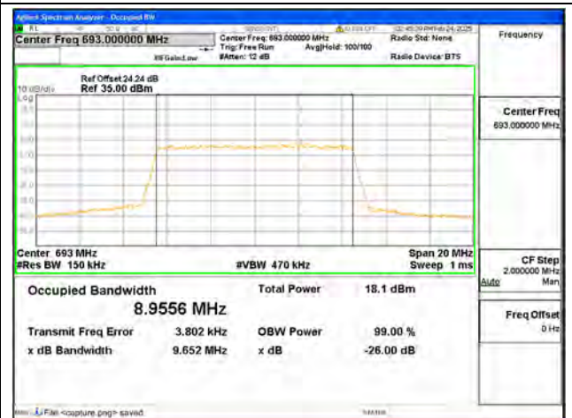
B71 / 10MHz / 256QAM/ High CH
