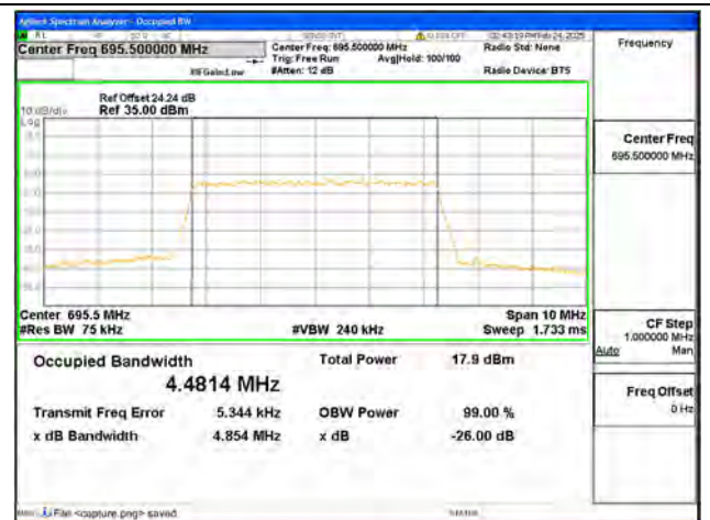
B71 / 5MHz / 256QAM/ High CH
