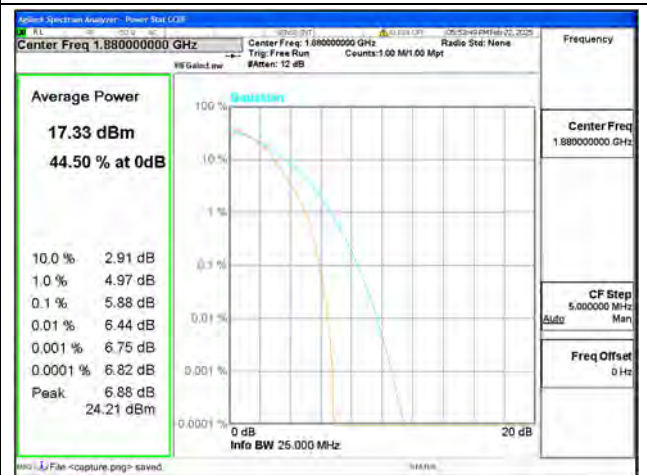
B2 / 15MHz / Mid CH / 16QAM
