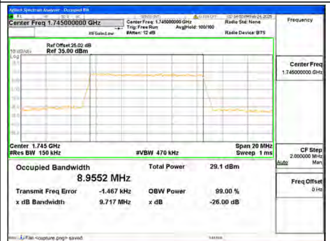
B66 / 10MHz / 16QAM/ Mid CH
