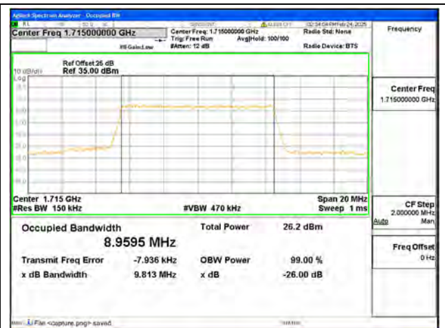
B66 / 10MHz / 16QAM/ Low CH
