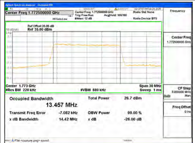
B66 / 15MHz / 16QAM/ High CH
