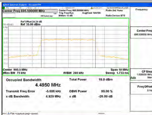
B71 / 5MHz / 64QAM/ High CH
