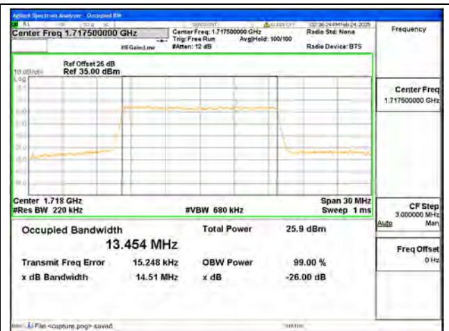
B66 / 15MHz / 16QAM/ Low CH
