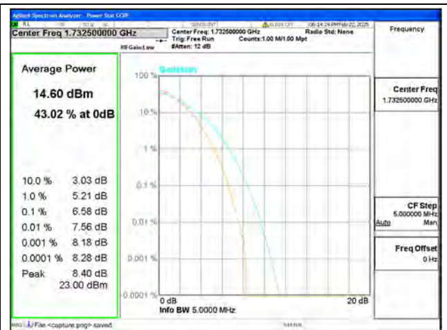
B4 / 5MHz / Mid CH / 256QAM
