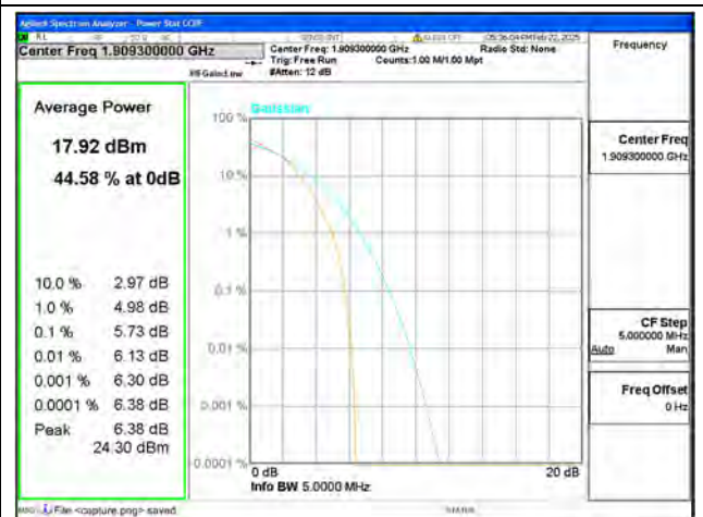
B2 / 1.4MHz / High CH / 16QAM
