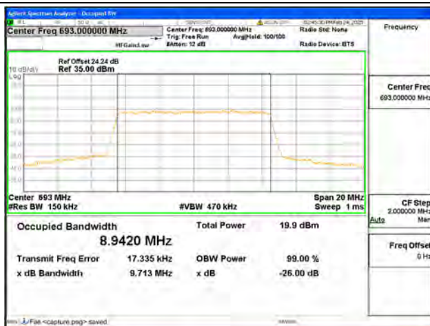
B71 / 10MHz / 64QAM/ High CH
