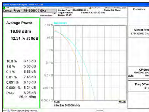
B4 / 1.4MHz / High CH / 64QAM
