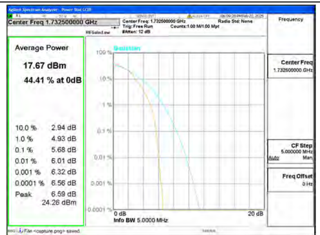
B4 / 3MHz / Mid CH / 16QAM
