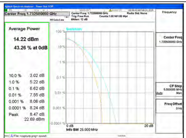
B4 / 15MHz / Mid CH / 256QAM
