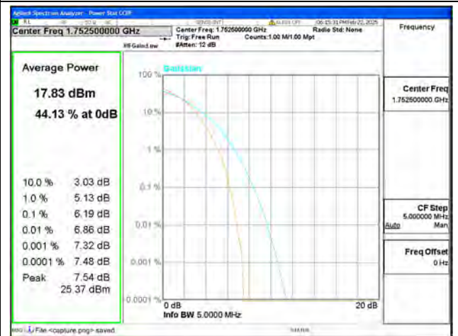
B4 / 5MHz / High CH / 16QAM
