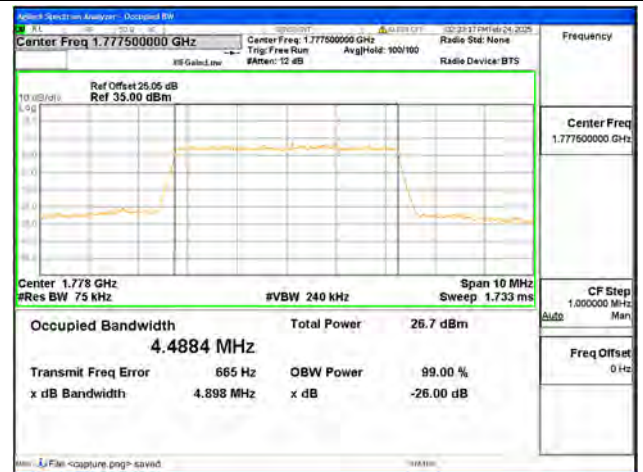
B66 / 5MHz / 16QAM/ High CH
