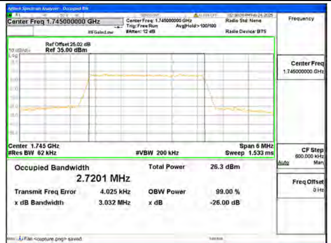
B66 / 3MHz / 16QAM/ Mid CH
