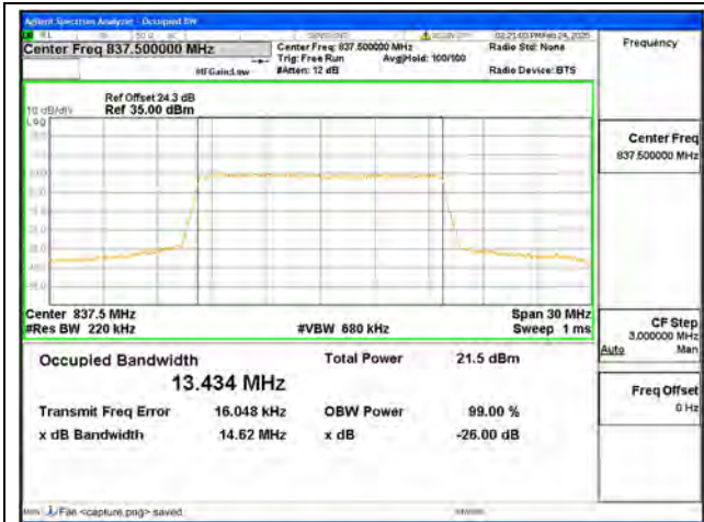
B19 / 15MHz / 64QAM/ Mid CH
