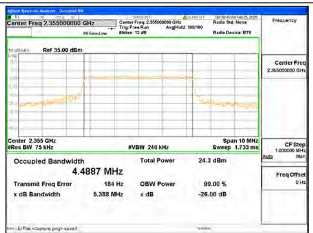
B40-2 / 5MHz / 256QAM/ Mid CH
