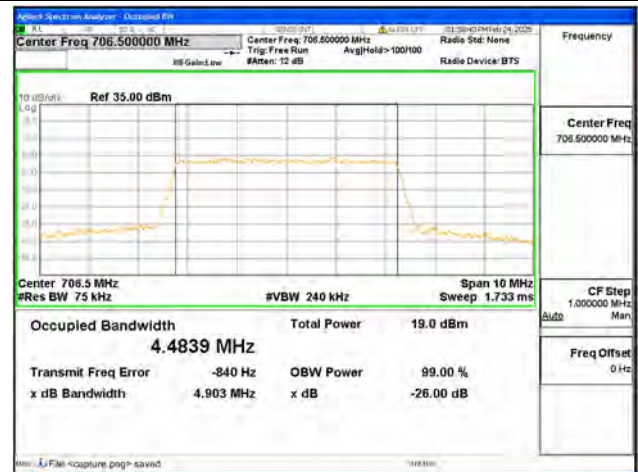
B17 / 5MHz / 256QAM/ Low CH
