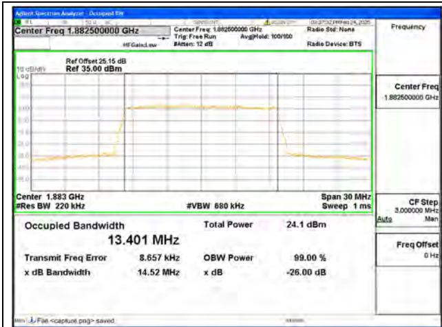
B25 / 15MHz / 64QAM/ Mid CH
