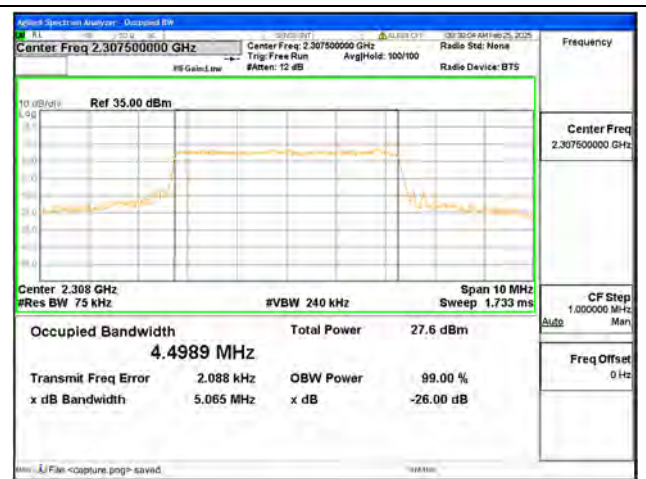
B40-1 / 5MHz / 16QAM/ Low CH
