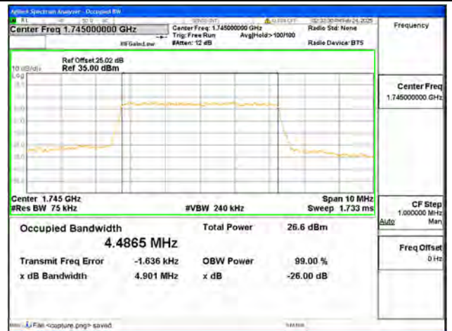
B66 / 5MHz / 16QAM/ Mid CH
