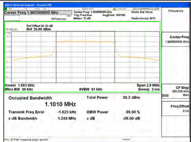
B25 / 1.4MHz / 16QAM/ Mid CH
