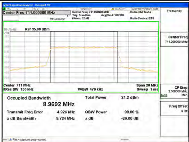
B17 / 10MHz / 64QAM/ High CH
