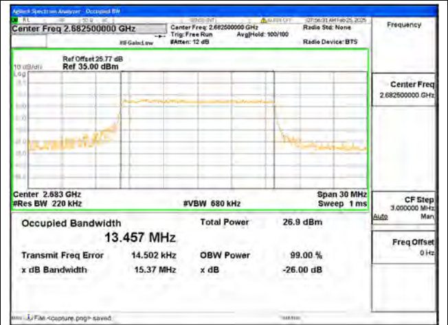
B41 / 15MHz / 16QAM/ High CH
