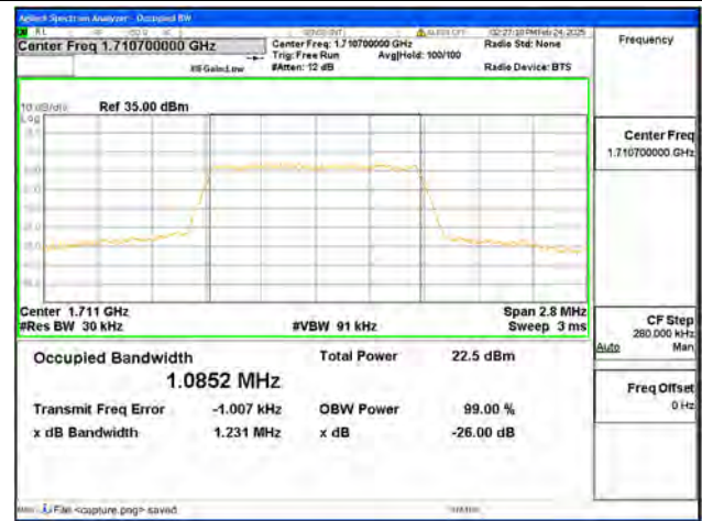
B66 / 1.4MHz / 256QAM/ Low CH
