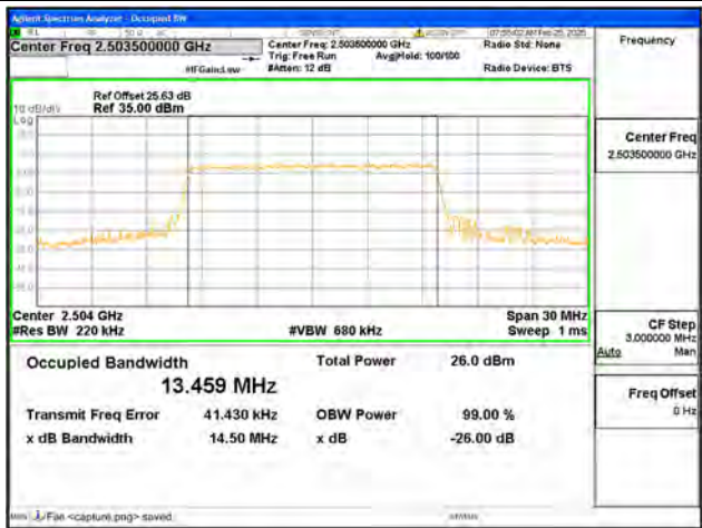
B41 / 15MHz / 64QAM/ Low CH
