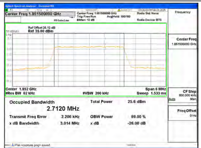
B25 / 3MHz / 16QAM/ Low CH
