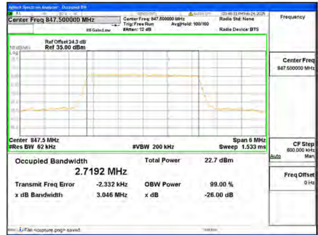
B26 / 3MHz / 16QAM/ High CH
