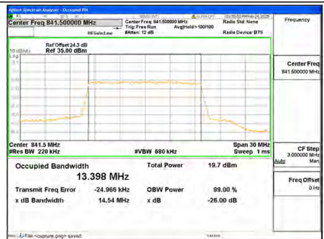
B26 / 15MHz / 256QAM/ High CH
