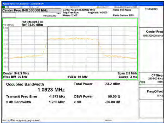
B26 / 1.4MHz / QPSK/ High CH
