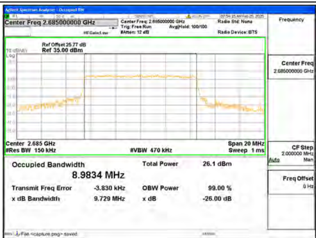
B41 / 10MHz / 64QAM/ High CH
