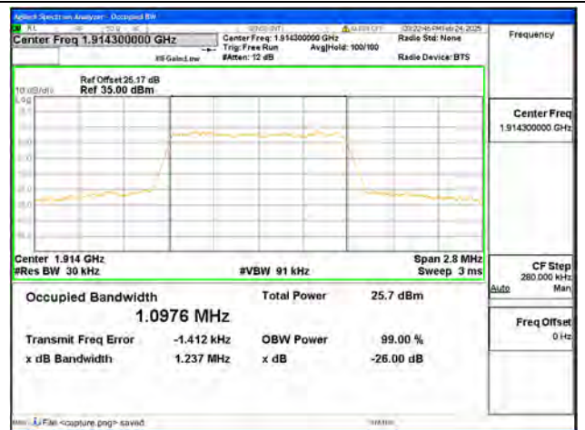
B25 / 1.4MHz / 16QAM/ High CH
