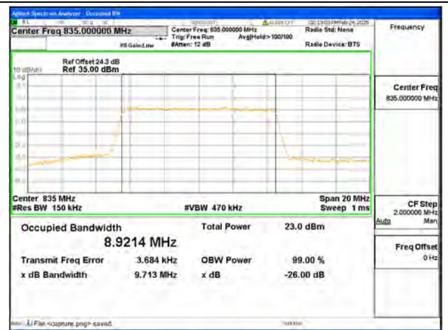
B19 / 10MHz / 16QAM/ Low CH
