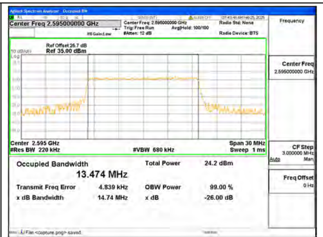
B38 / 15MHz / 256QAM/ Mid CH
