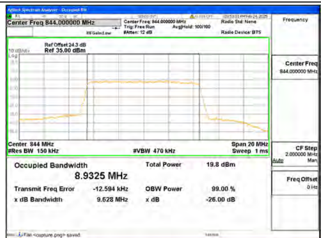
B26 / 10MHz / 256QAM/ High CH
