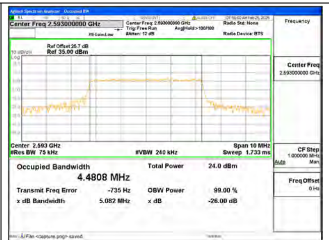
B41 / 5MHz / 256QAM/ Mid CH
