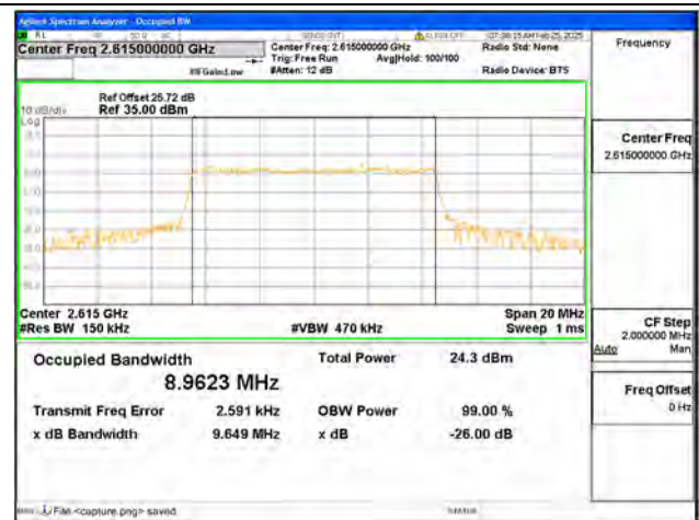
B38 / 10MHz / 256QAM/ High CH
