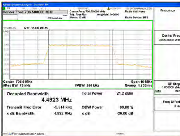
B17 / 5MHz / 64QAM/ Low CH
