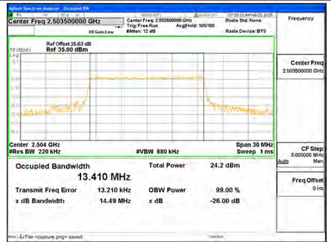
B41 / 15MHz / 256QAM/ Low CH
