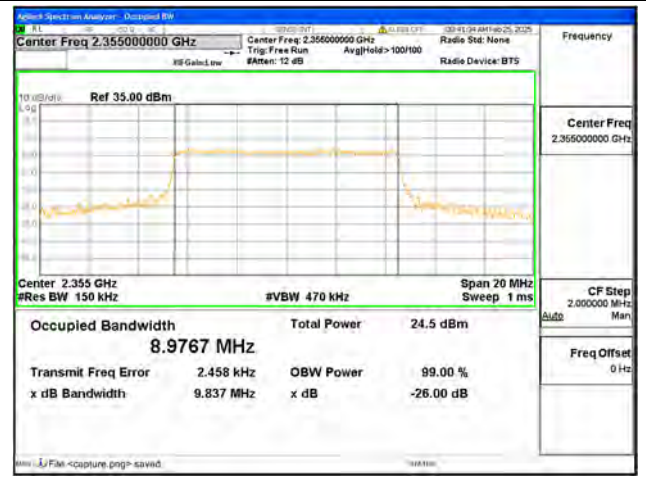
B40-2 / 10MHz / 256QAM / Mid CH
