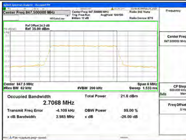
B26 / 3MHz / 64QAM/ High CH
