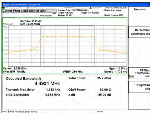
B41 / 5MHz / 64QAM/ High CH
