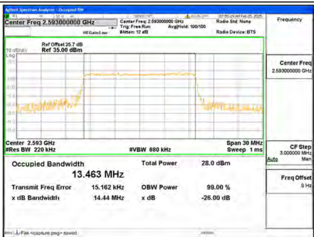
B41 / 15MHz / QPSK/ Mid CH
