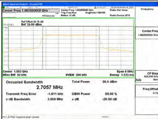
B25 / 3MHz / QPSK/ Mid CH
