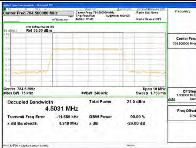
B13 / 5MHz / 64QAM/ High CH
