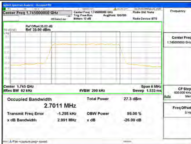
B66 / 3MHz / QPSK/ Mid CH
