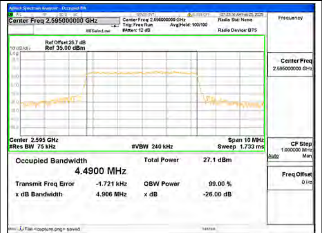
B38 / 5MHz / 16QAM/ Mid CH
