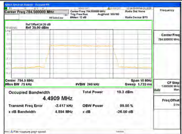
B13 / 5MHz / 256QAM/ High CH
