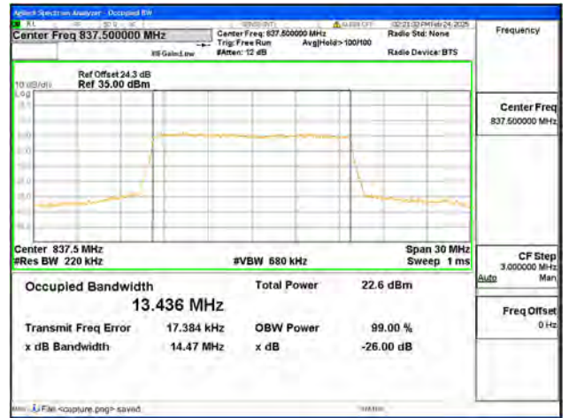
B19 / 15MHz / 16QAM/ High CH
