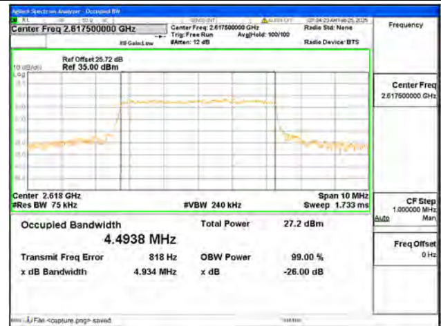
B38 / 5MHz / 16QAM/ High CH
