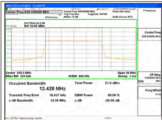
B26 / 15MHz / 64QAM/ Mid CH
