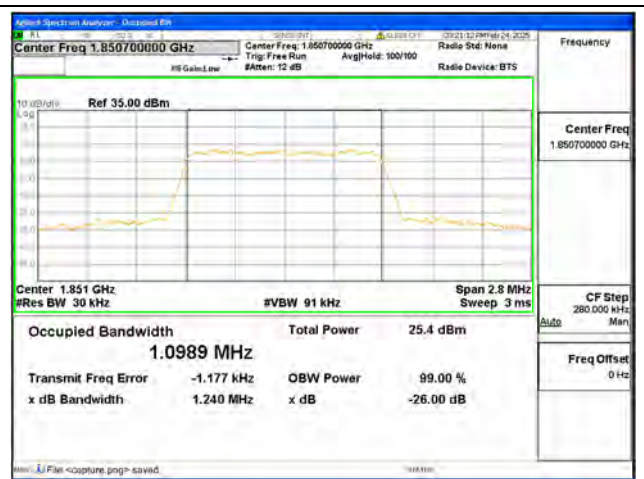
B25 / 1.4MHz / 16QAM/ Low CH
