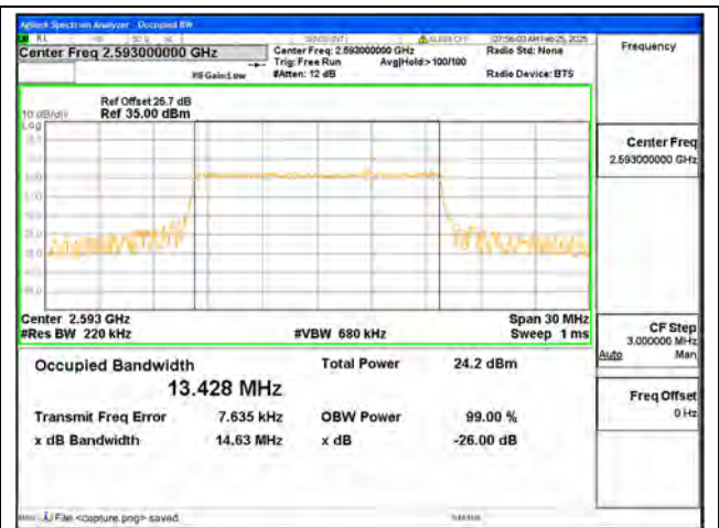
B41 / 15MHz / 256QAM/ Mid CH
