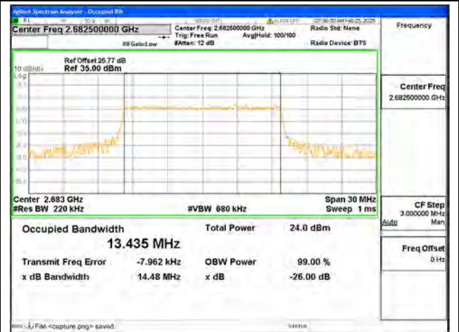
B41 / 15MHz / 256QAM/ High CH
