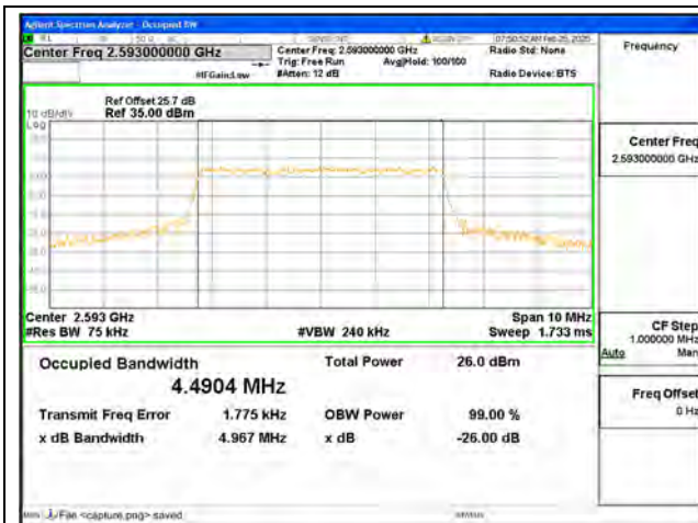
B41 / 5MHz / 64QAM/ Mid CH
