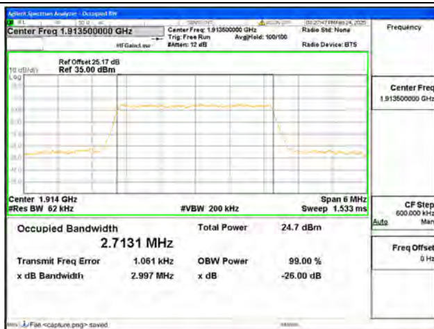
B25 / 3MHz / 64QAM/ High CH
