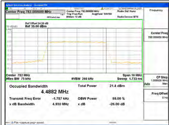
B13 / 5MHz / 64QAM/ Mid CH
