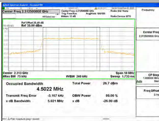
B40-1 / 5MHz / 64QAM/ High CH
