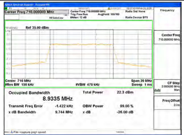
B17 / 10MHz / 16QAM/ Mid CH
