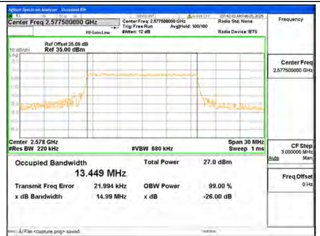
B38 / 15MHz / 16QAM/ Low CH
