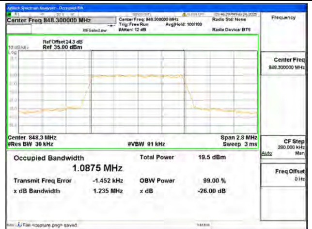
B26 / 1.4MHz / 256QAM/ High CH
