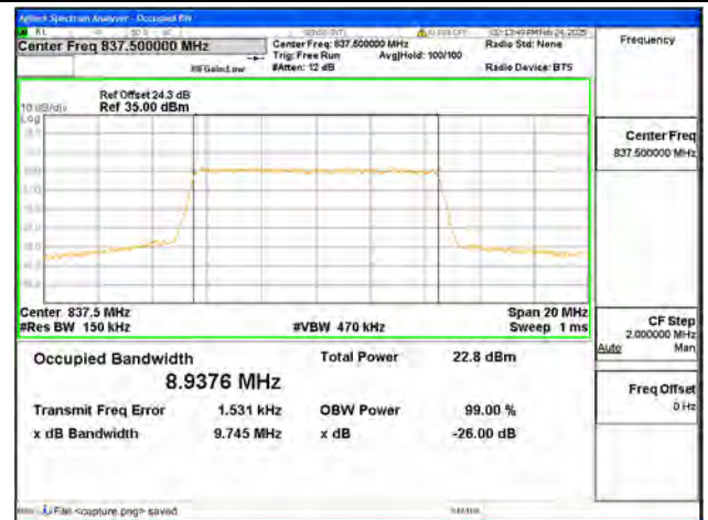
B19 / 10MHz / 16QAM/ Mid CH
