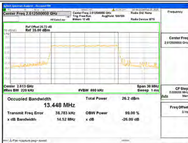
B38 / 15MHz / 64QAM/ High CH
