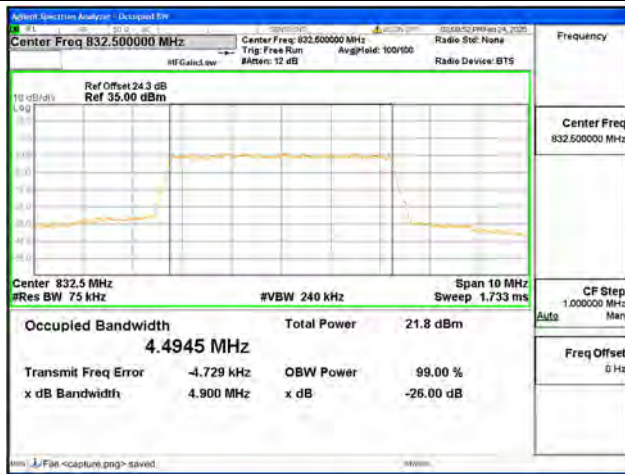
B19 / 5MHz / 64QAM/ Low CH
