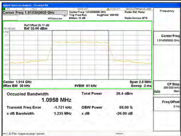
B25 / 1.4MHz / QPSK/ High CH
