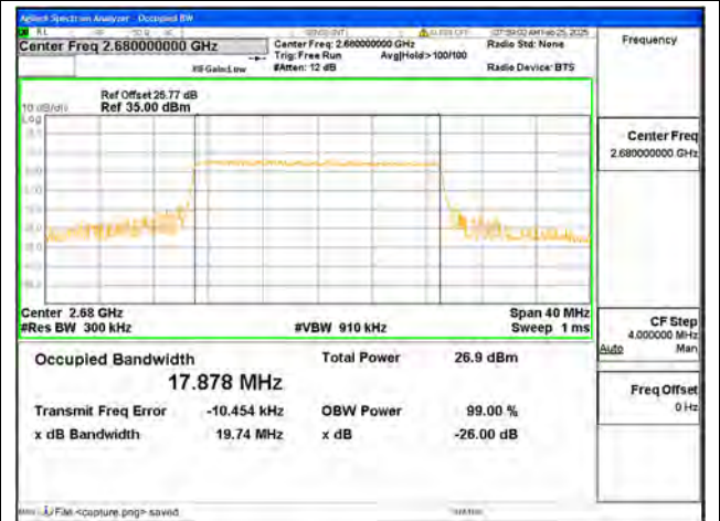
B41 / 20MHz / 16QAM/ High CH
