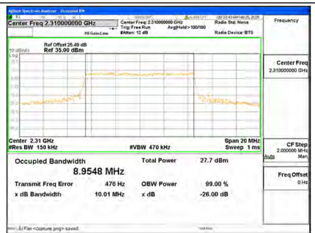
B40-1 / 10MHz / 16QAM / Mid CH
