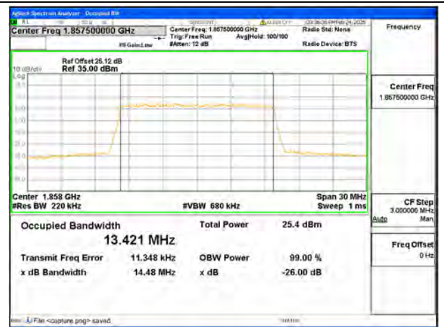
B25 / 15MHz / 16QAM/ Low CH
