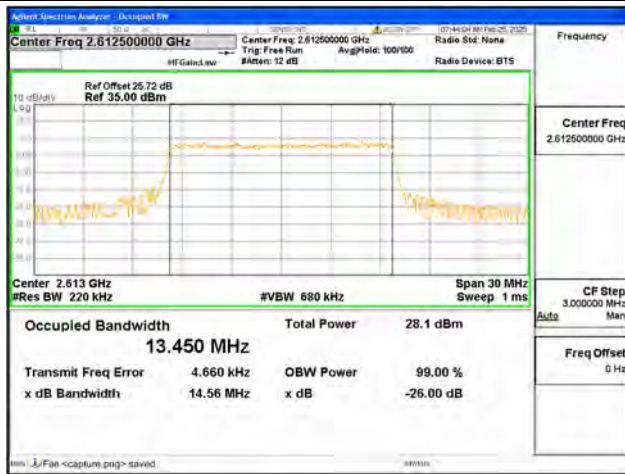
B38 / 15MHz / QPSK/ High CH
