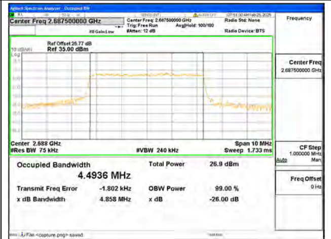
B41 / 5MHz / 16QAM/ High CH
