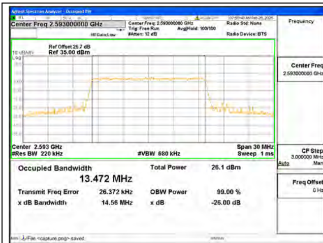
B41 / 15MHz / 64QAM/ Mid CH
