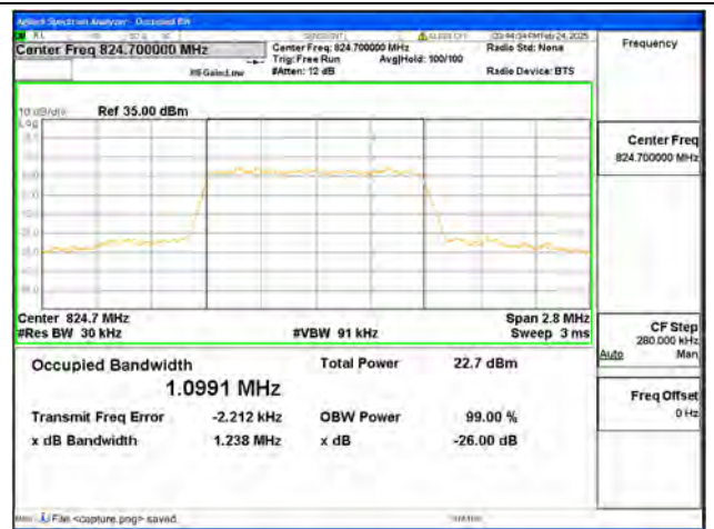
B26 / 1.4MHz / 16QAM/ Low CH
