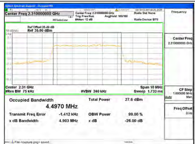
B40-1 / 5MHz / 16QAM/ Mid CH
