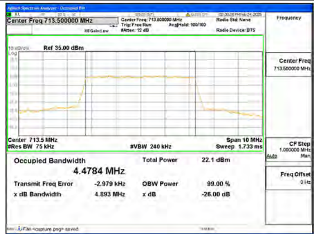
B17 / 5MHz / 16QAM/ High CH
