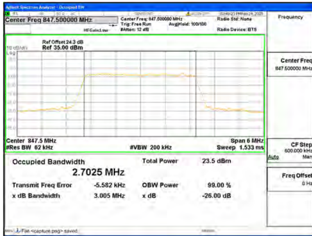
B26 / 3MHz / QPSK/ High CH
