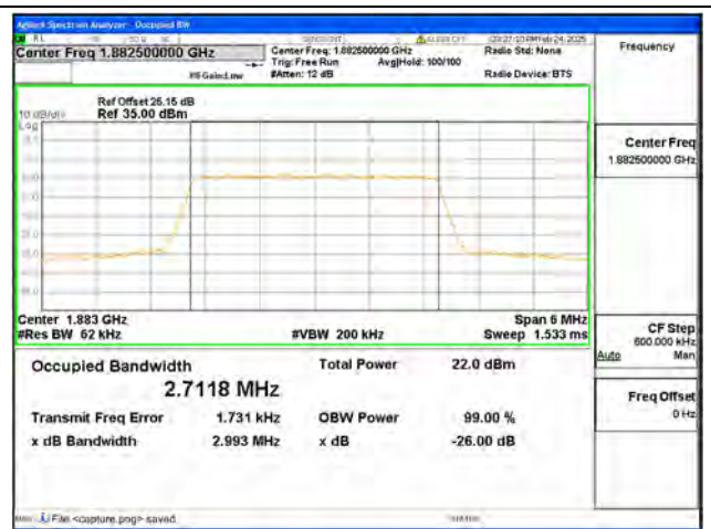
B25 / 3MHz / 256QAM/ Mid CH
