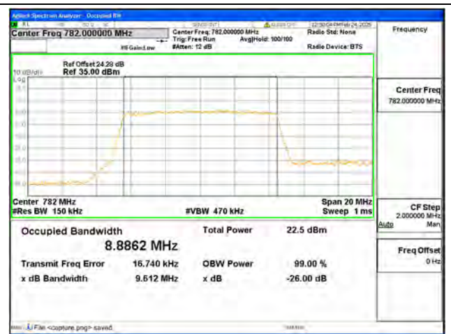
B13 / 10MHz / 16QAM/ Mid CH
