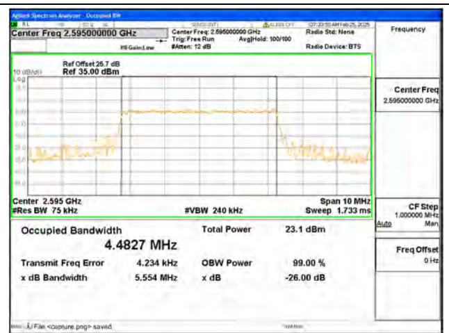
B38 / 5MHz / 256QAM/ Mid CH
