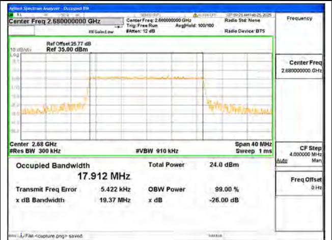
B41 / 20MHz / 256QAM/ High CH
