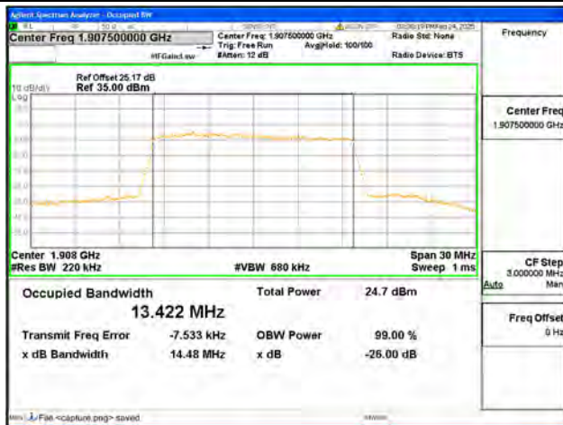
B25 / 15MHz / 64QAM/ High CH
