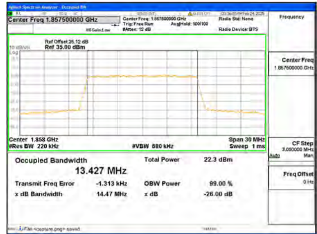
B25 / 15MHz / 256QAM/ Low CH
