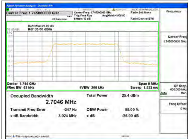
B66 / 3MHz / 64QAM/ Mid CH
