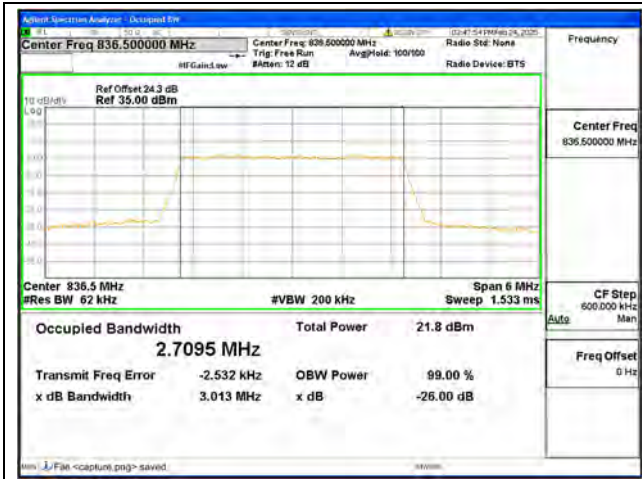
B26 / 3MHz / 64QAM/ Mid CH
