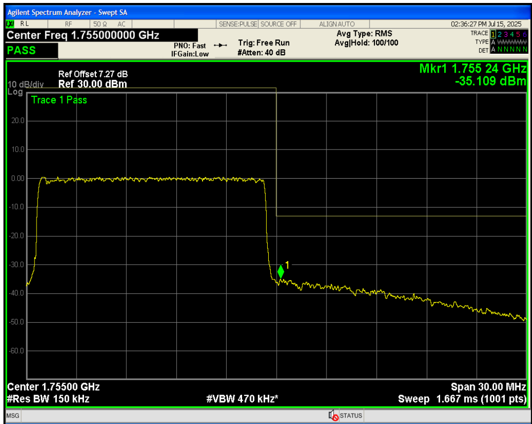
Band4 QAM16 BW=20MHz Channel=20050 RB Size=100 Position=#0
