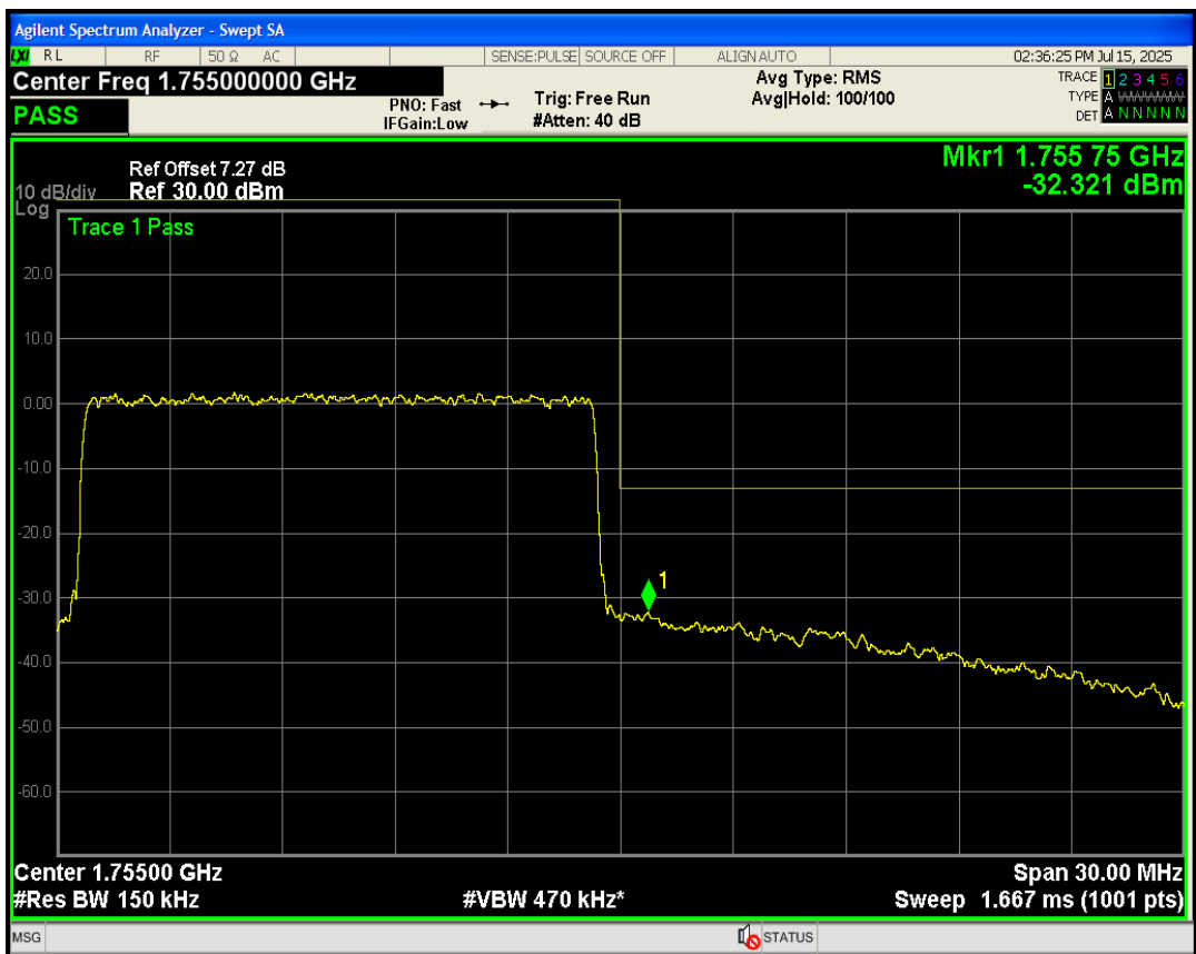
Band4 QAM16 BW=15MHz Channel=20325 RB Size=75 Position=#0
