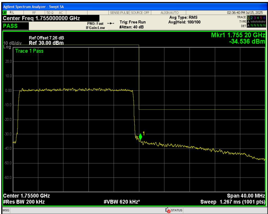
Band4 QAM16 BW=20MHz Channel=20300 RB Size=100 Position=#0
