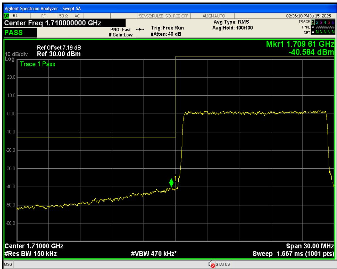
Band4 QAM16 BW=15MHz Channel=20025 RB Size=75 Position=#0
