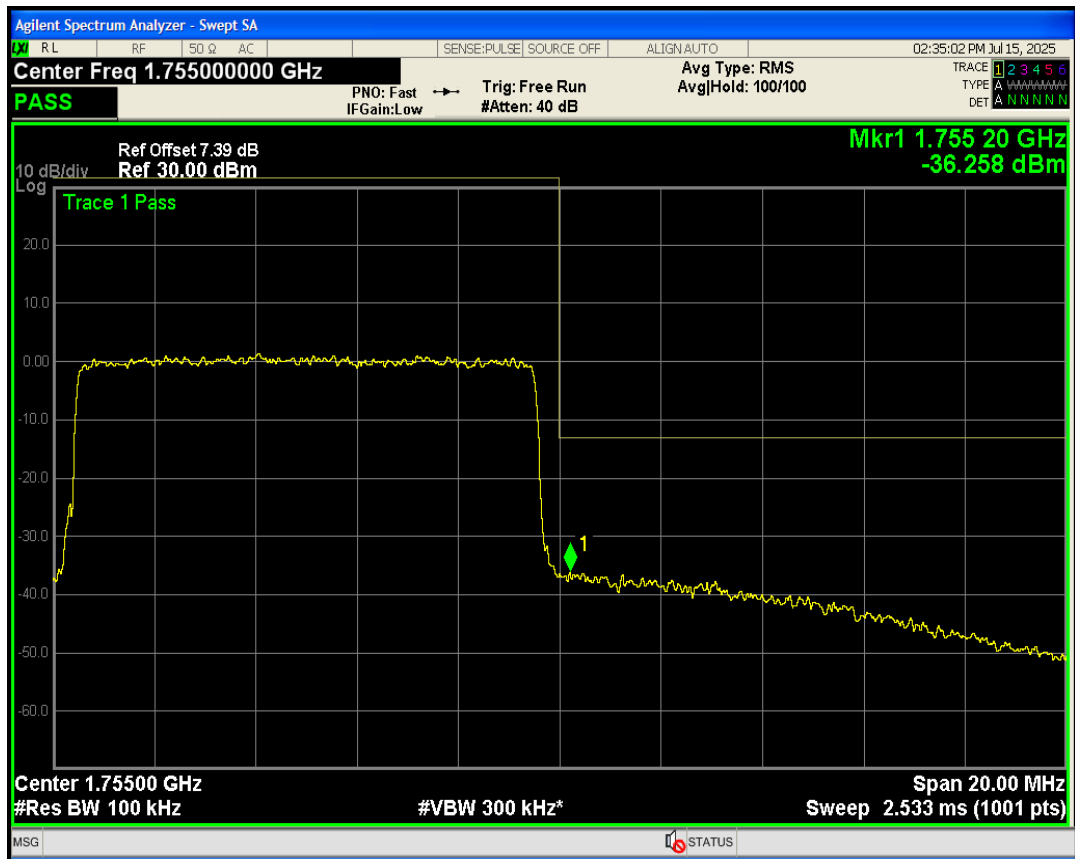
Band4 QPSK BW=15MHz Channel=20025 RB Size=75 Position=#0
