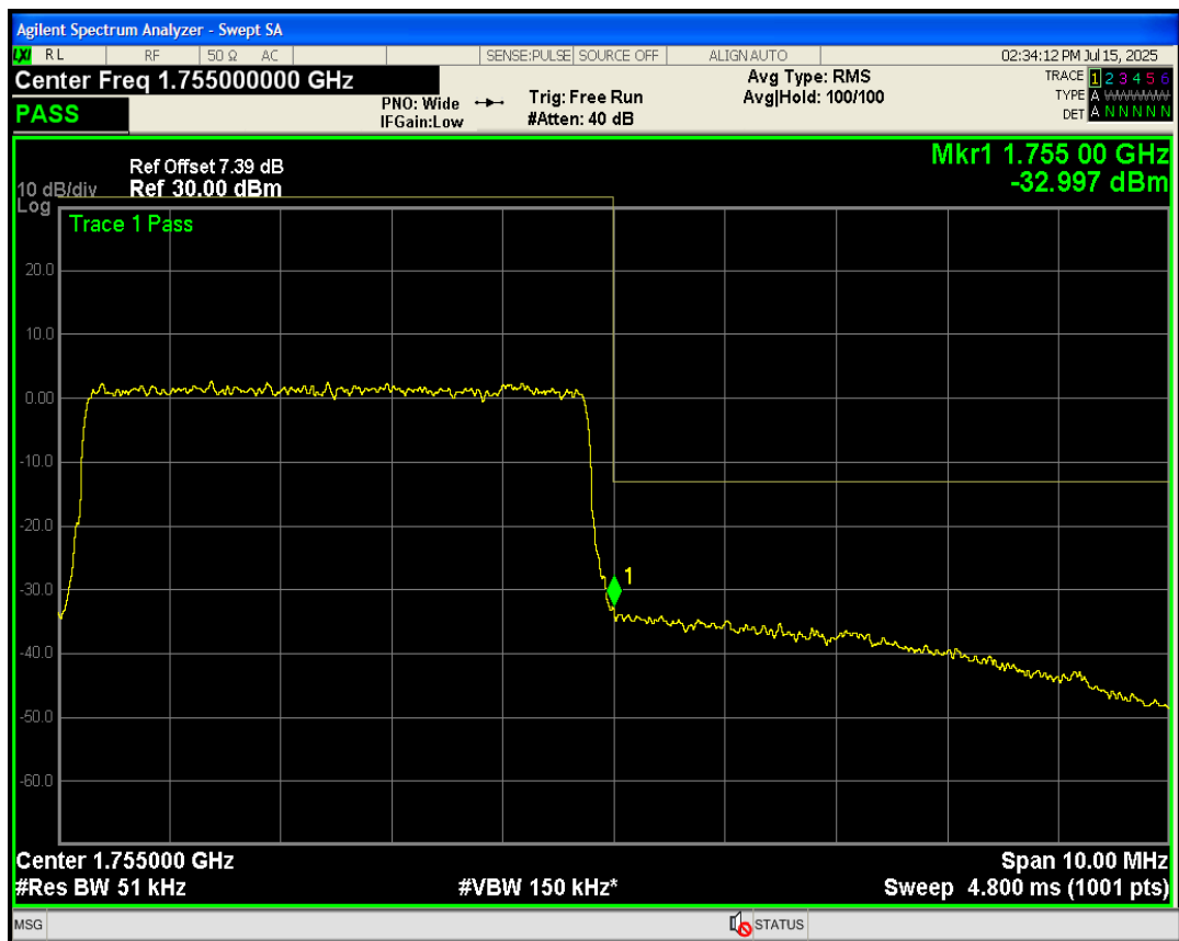
Band4 QAM16 BW=5MHz Channel=20375 RB Size=25 Position=#0
