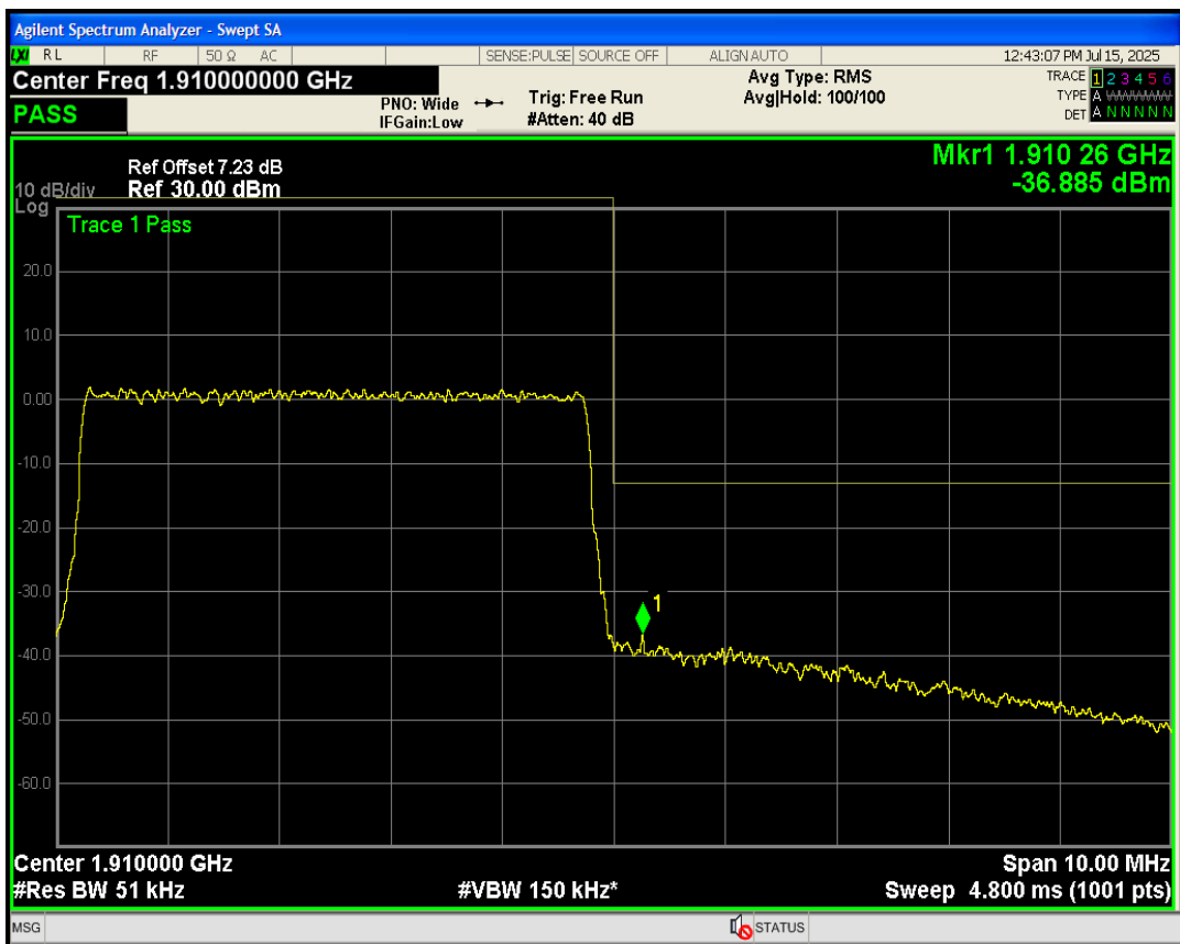
Band2 QPSK BW=5MHz Channel=19175 RB Size=25 Position=#0
