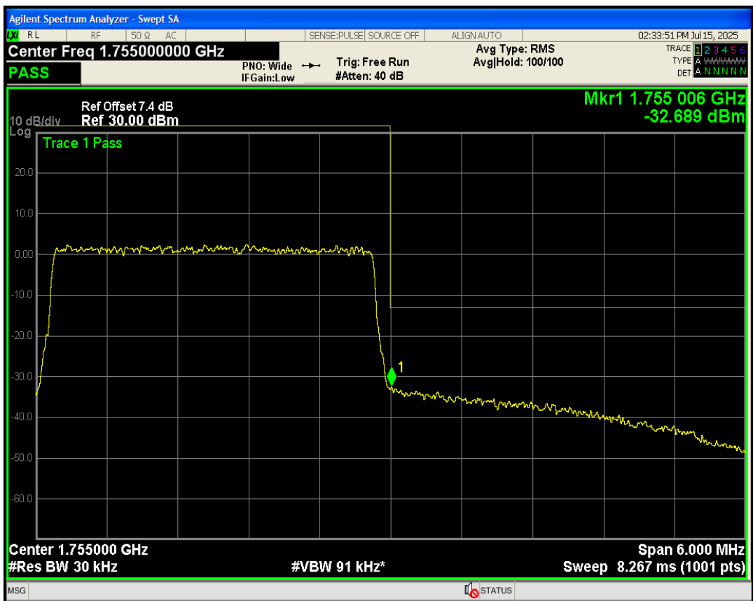
Band4 QAM16 BW=3MHz Channel=20385 RB Size=15 Position=#0
