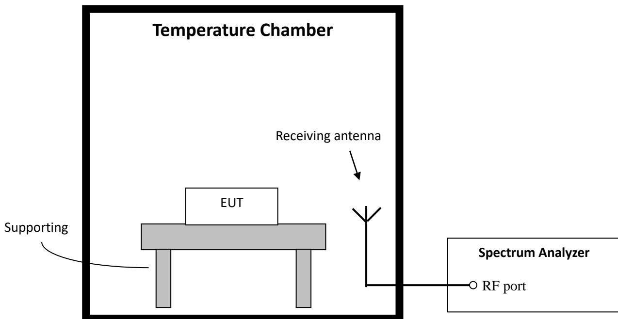
**TEST REPORT****5.3 Test procedure and test setup**
