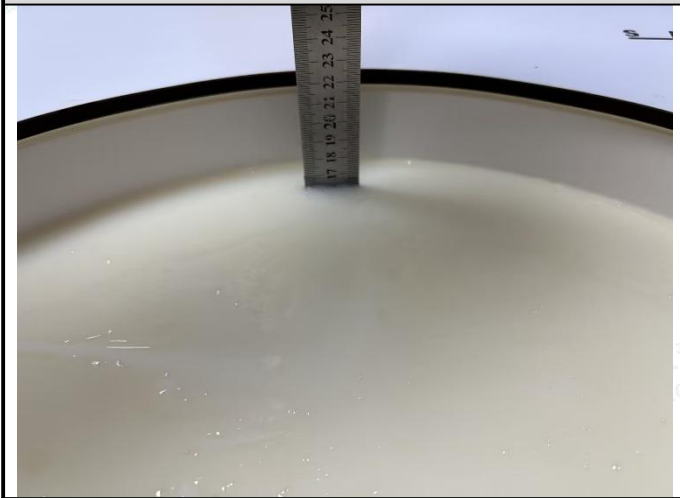
Photo 1: Tissue Simulant Liquid for Head 700-3000Mhz
