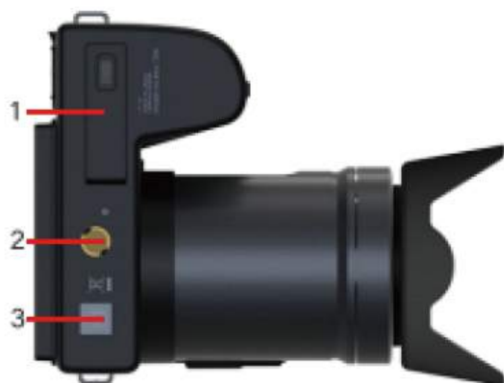
1:Battery Door 2:Tripod slot 3:Memory slot
