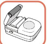
Load paper ensuring that the end of the roll is facing the front of the device.
