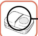
Close the device with the end of the sticker roll pulled through the opening.
