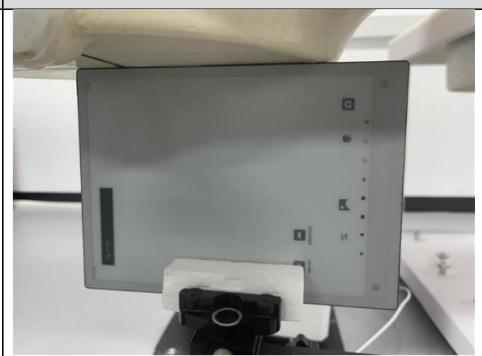
A photograph showing the right side of the EUT at 0mm offset. The EUT is mounted on a white stand. A large, light-colored cylindrical probe or antenna is positioned above the EUT. The background includes a white wall and some equipment on a table. |
