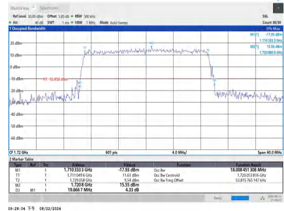
Band4-20MHz-16QAM-20050-100RB#0-PASS
