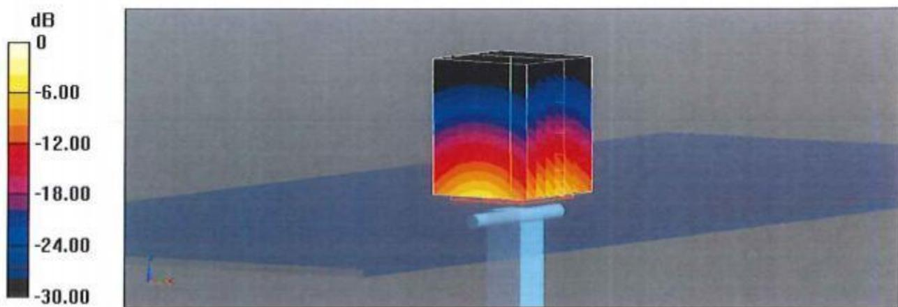
$$0 \text{ dB} = 12.8 \text{ W/kg} = 11.07 \text{ dBW/kg}$$
