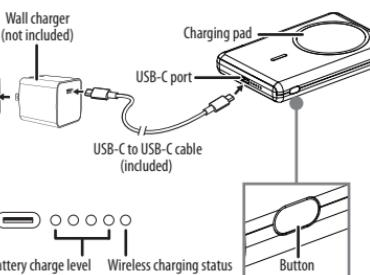
The indicator LEDs light to indicate the current charge level:
