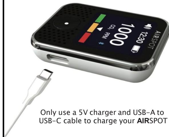
Only use a 5V charger and USB-A to USB-C cable to charge your AIRSPOT
