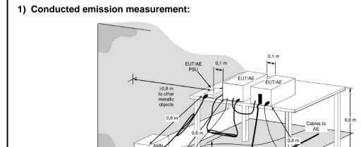
AMNs or AANs bonded to a reference ground plane
