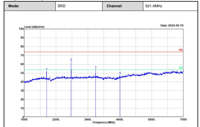
Project No. : 2405V28082E Test Mode : Transmitting Test Voltage : Power by battery Environment : 23.7%/62%R.H./99.8kPa
