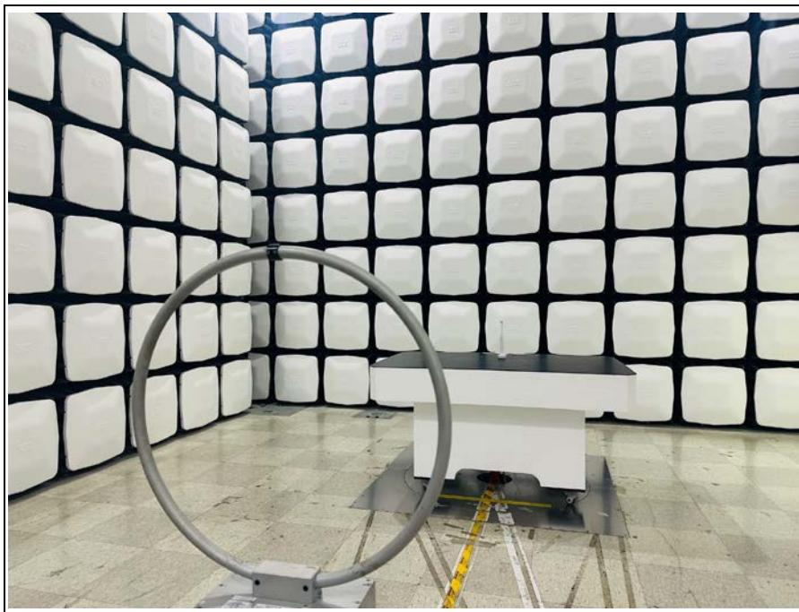
**3. Photo of Radiated Spurious Emission Test (30 MHz ~ 1 000 MHz)**
