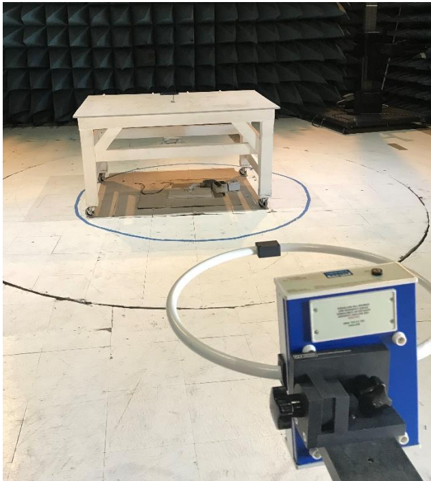
RE Test Setup – Active Loop Antenna (9 KHz to 30 MHz) Vertical and Horizontal Polarization
