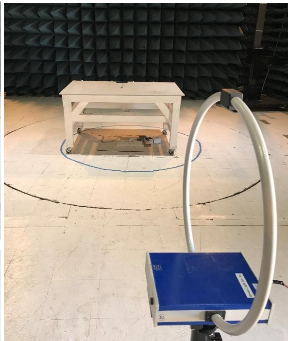
RE Test Setup – Active Loop Antenna (9 KHz to 30 MHz) Vertical and Horizontal Polarization
