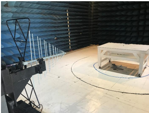
RE Test Setup – BiLog Antenna (30 MHz to 1 GHz) Vertical and Horizontal Polarization
