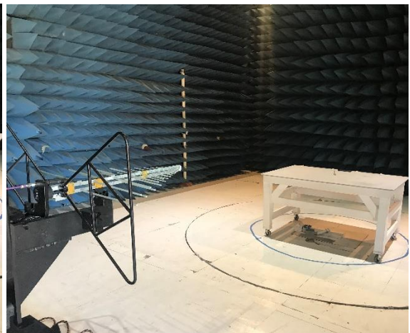
RE Test Setup – BiLog Antenna (30 MHz to 1 GHz) Vertical and Horizontal Polarization
