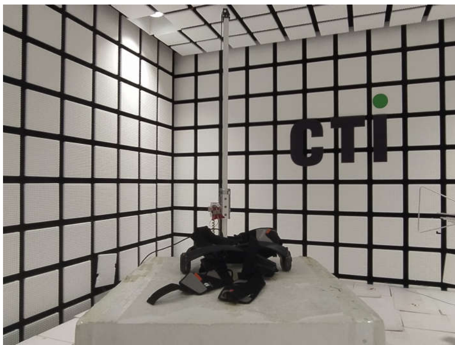
Radiated spurious emission Test Setup-2(Above 1GHz)
