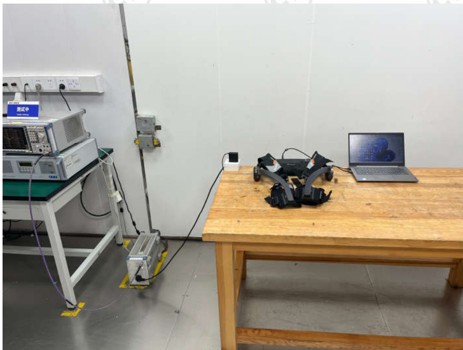
Conducted Emissions Test Setup
