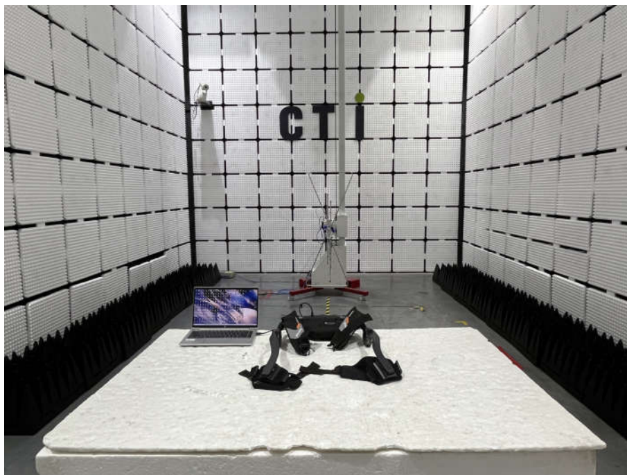
Radiated spurious emission Test Setup-1(Below 1GHz)
