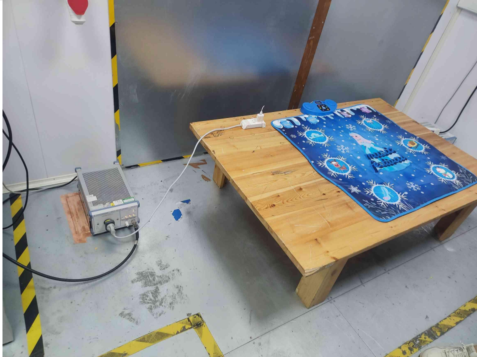
Conducted emissions at AC power line (150kHz-30MHz)
