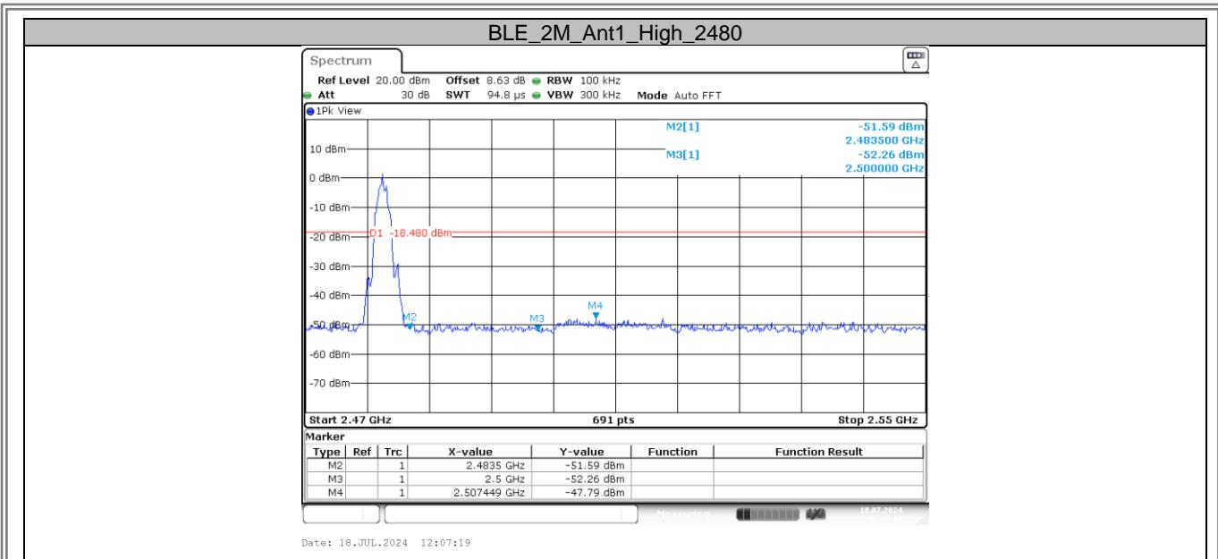
**APPENDIX G POWER SPECTRAL DENSITY****Power Spectral Density**
