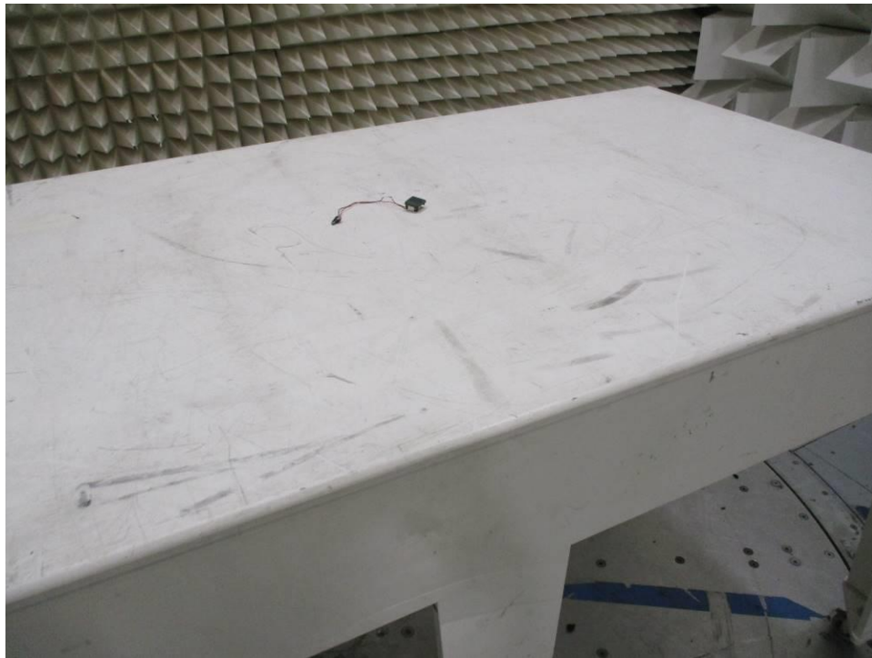
Figure 0-18 Radiated Emissions Test Setup Earpiece Battery Mode 30 MHz-1 GHz
