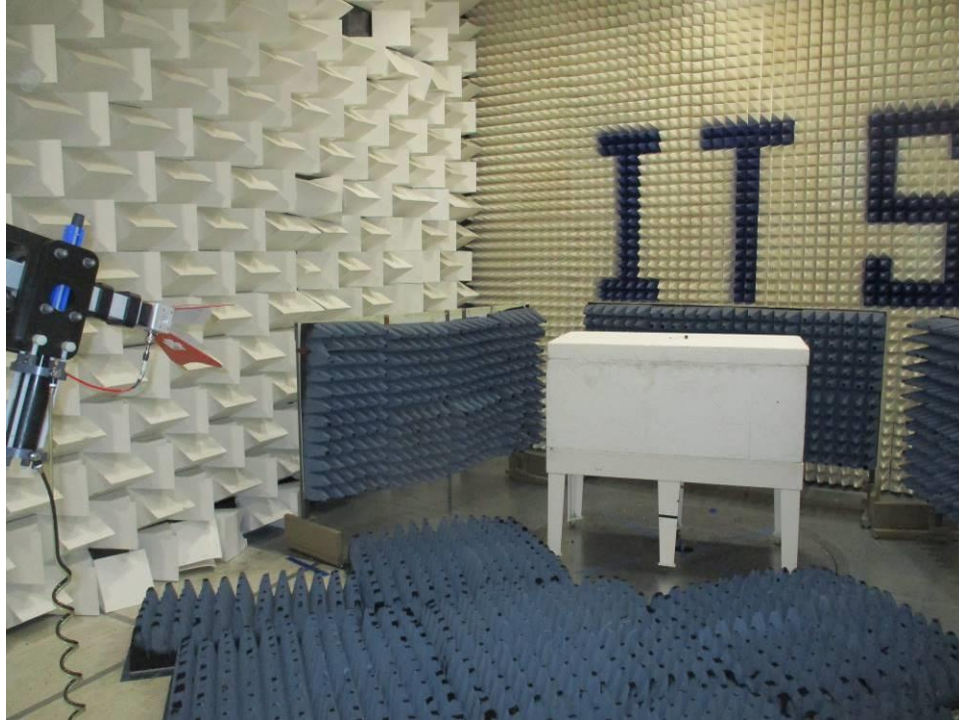
Figure 0-11 Radiated Spurious Emissions Test Setup Earpiece Battery Mode 1 GHz-18 GHz
