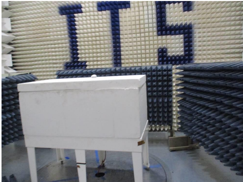
Figure 0-16 Radiated Spurious Emissions Test Setup Charging Mode 1 GHz-18 GHz
