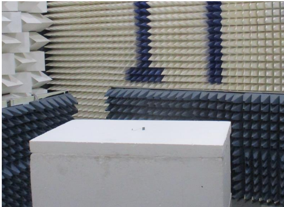
Figure 0-12 Radiated Spurious Emissions Test Setup Earpiece Battery Mode 1 GHz-18 GHz
