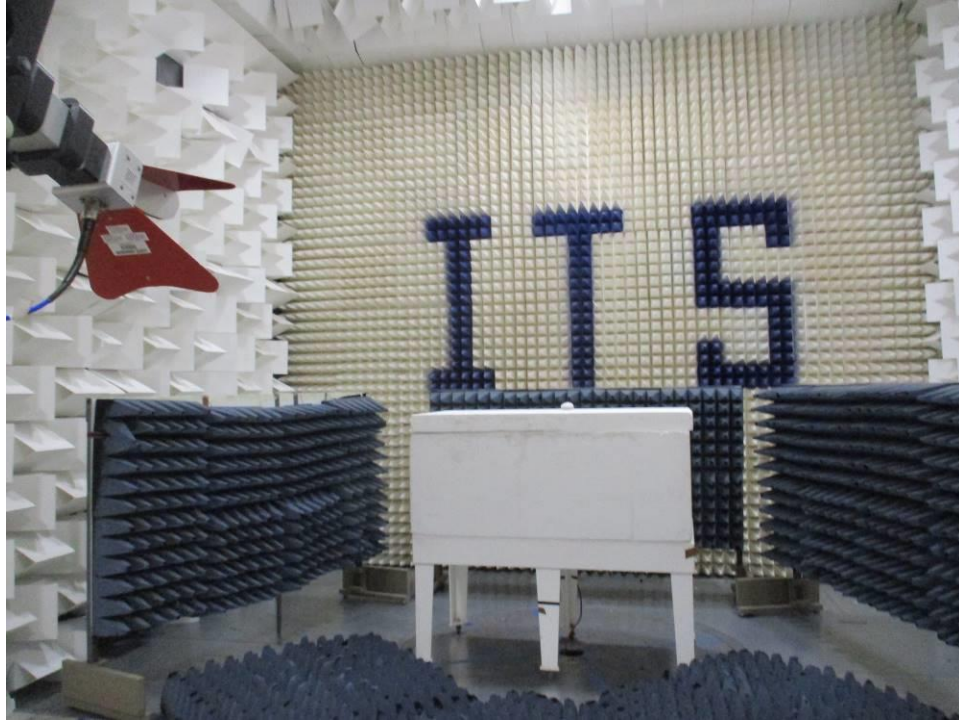
Figure 0-15 Radiated Spurious Emissions Test Setup Charging Mode 1 GHz-18 GHz
