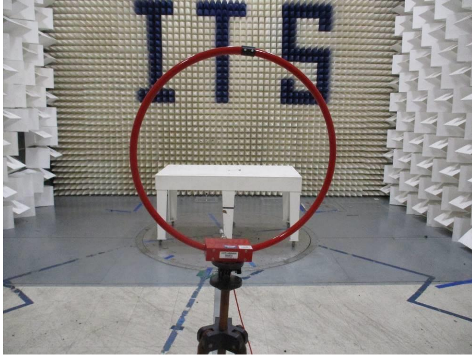
Figure 0-7 Radiated Spurious Emissions Test Setup Earpiece Battery Mode 9 kHz – 30 MHz X Axis
