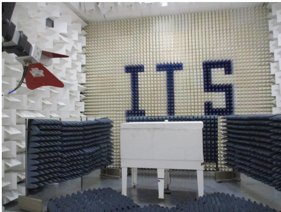
Figure 0-2 Band Edge Charging Mode Test Setup
