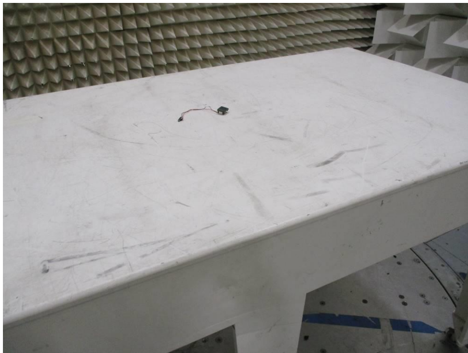
Figure 0-4 Radiated Spurious Emissions Test Setup Earpiece Battery Mode 30 MHz-1 GHz
