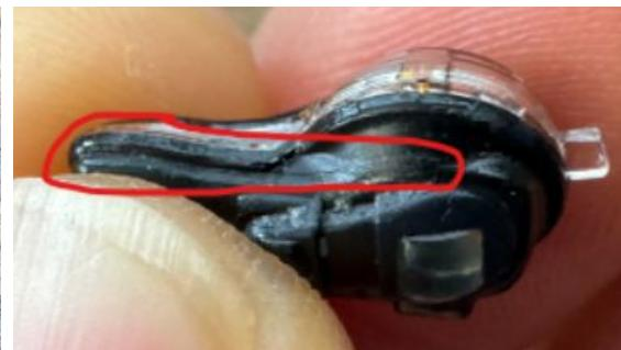
After the antenna is successfully etched onto the plastic housing, it is then coated with a layer of acrylic resin based paint. See paint covering circled in red above, where raised antenna is still slightly visible under the paint.
