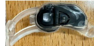
After the paint layer, the device is wrapped in a soft silicone jacket that flexibly adapts the earpiece to differently shaped ears.
