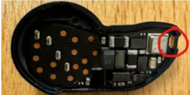
The LDS antenna conductor on the inside of the plastic housing is soldered directly to the PCBA to connect to the BLE chip.
