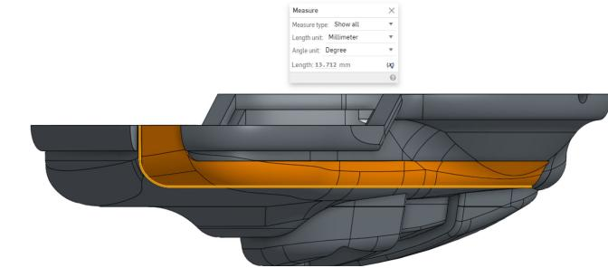
The length of the antenna is 12.9mm on the short length, and 13.7mm on the long side, for an average length of 13.4mm:
