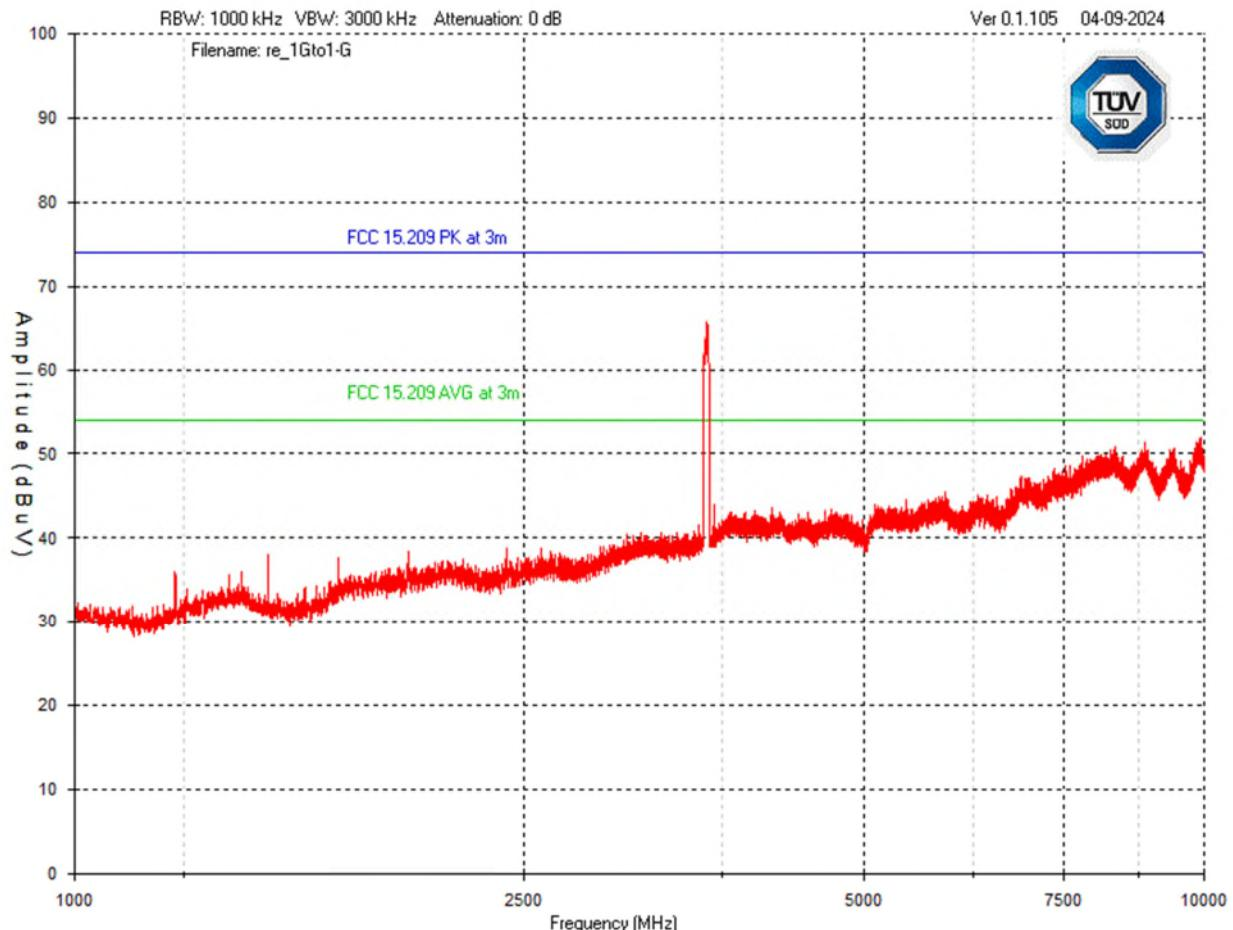
Note: Peak reading shown in graph above. Frequency shown above was the in-band signal due to RF leakage from the termination(s) used.
