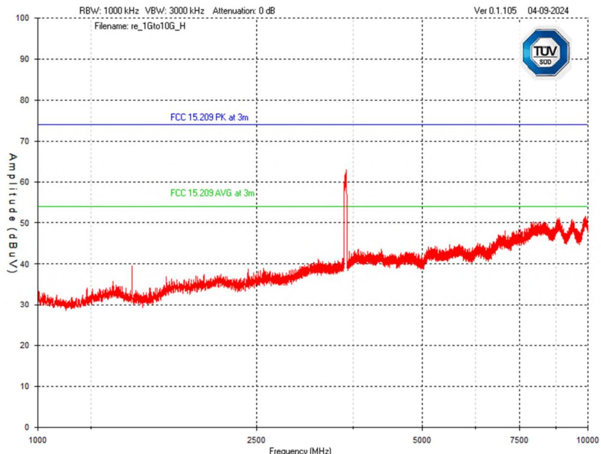
Note: Peak reading shown in graph above. Frequency shown above the was the in-band signal due to RF leakage from the termination(s) used.
