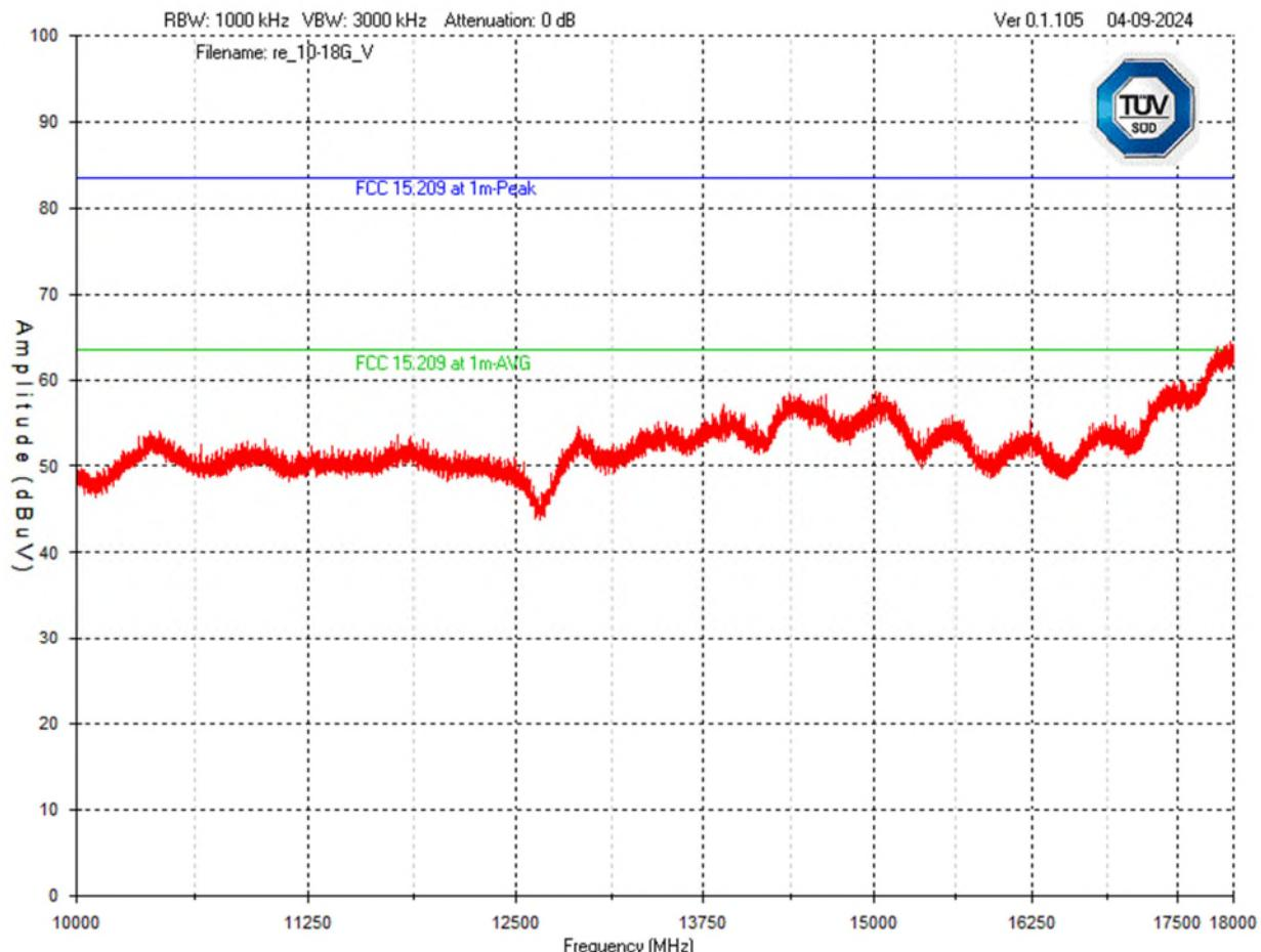
Note: Peak reading shown in graph above. Above 17.5 GHz, measurements to the AVG limit were verified with an average detector. No emissions were detected and the noise floor in average mode was below the average limit. The EUT was scanned to 40 GHz, no emissions were detected between 18 GHz and 40 GHz and the noise floor was below the applicable limit.
