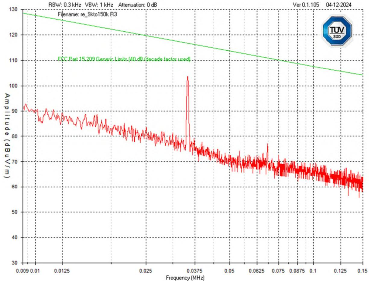
Note: Peak reading shown. Frequency at 35 kHz was determined to be an ambient emission, not related to EUT. No significant emission (i.e., less than 10dB below the limit) was noted.
