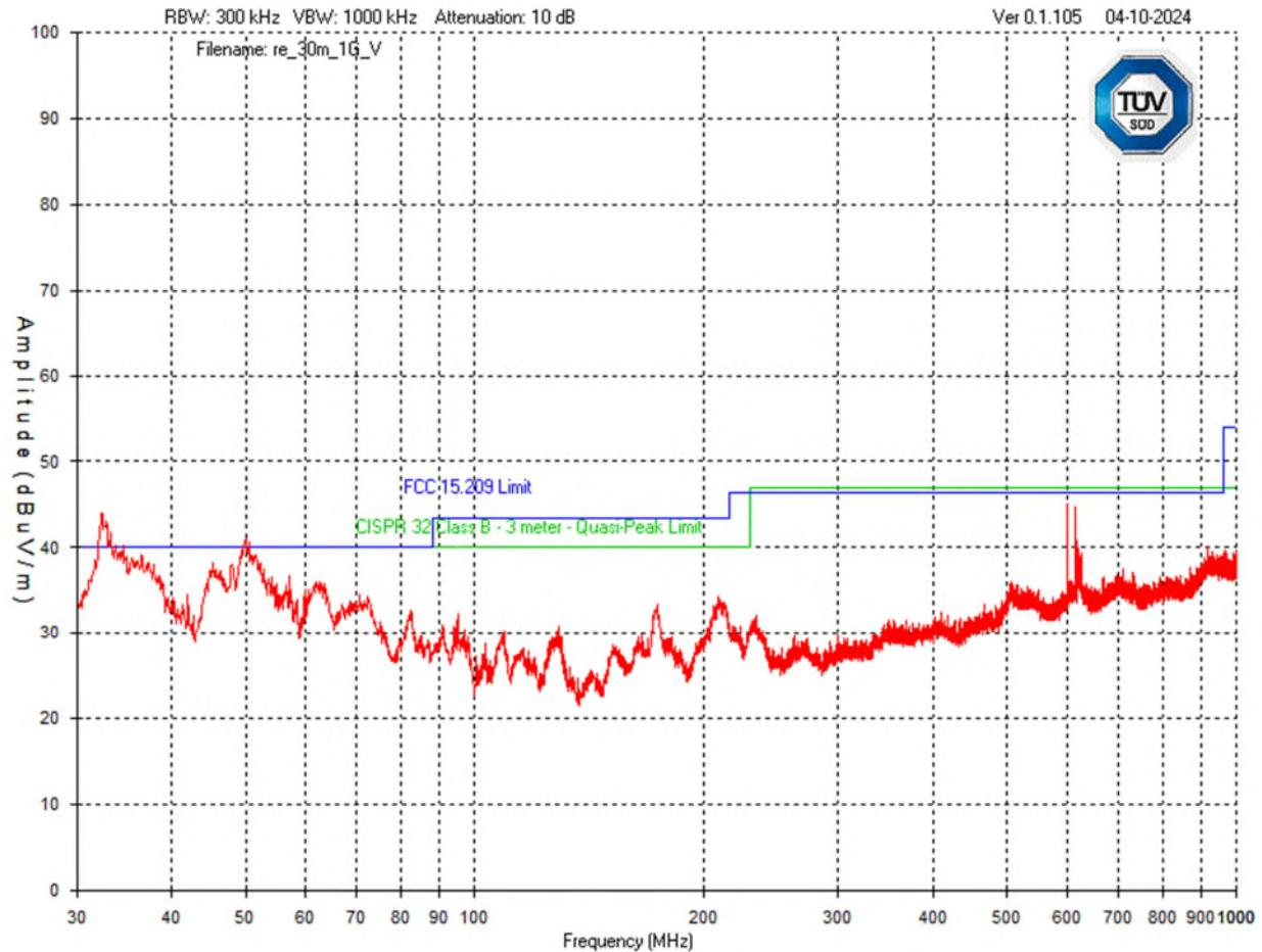
Note: Peak reading shown in graph above vs. Quasi-peak limit. Where the peak reading meets the quasi-peak limit, the EUT is determined to pass without requiring quasi-peak measurement.
