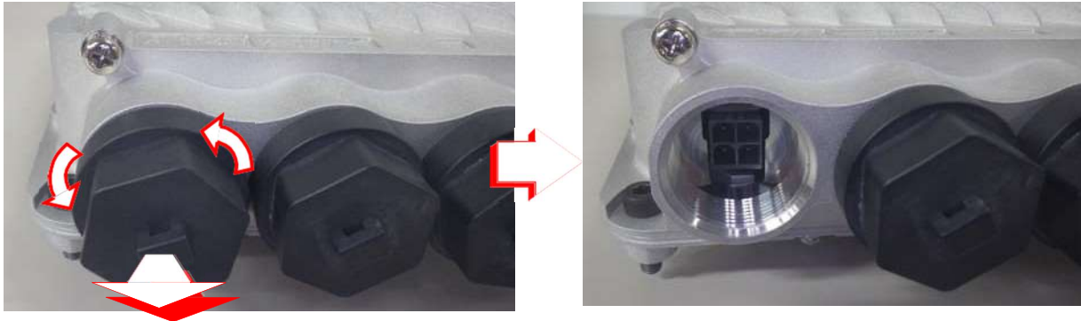
Figure 5-3 Remove the Protective Cap of the Power Port
