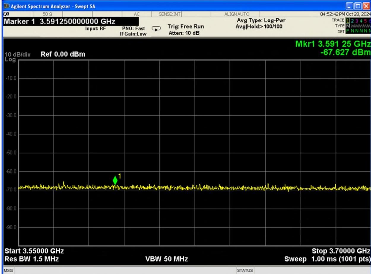
Domain Proxy Missing Required parameters (responseCode 102) was verified by logs. The EUT did not transmit.
