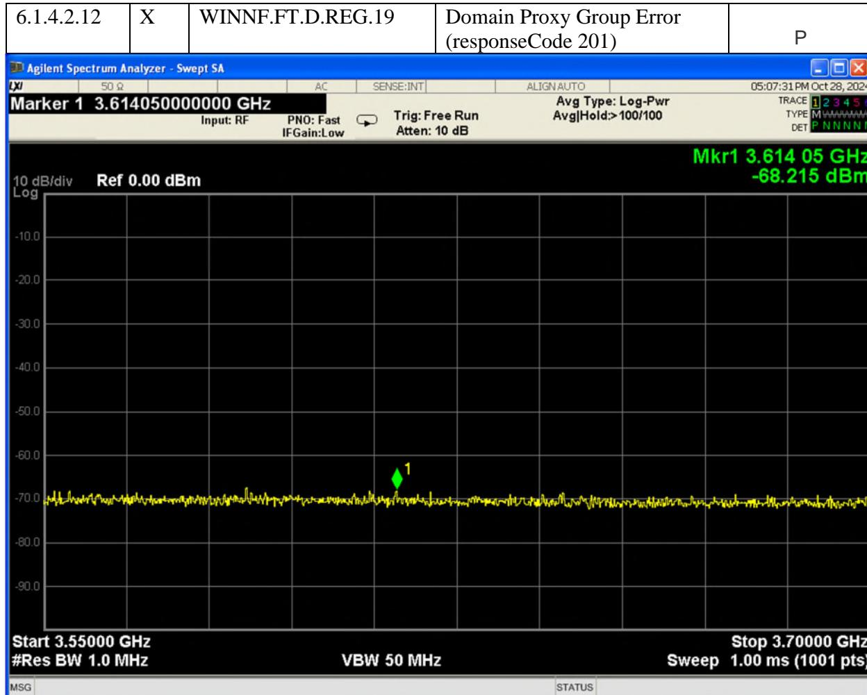
Domain Proxy Group Error (responseCode 201) was verified via logs. The EUT did not transmit.
