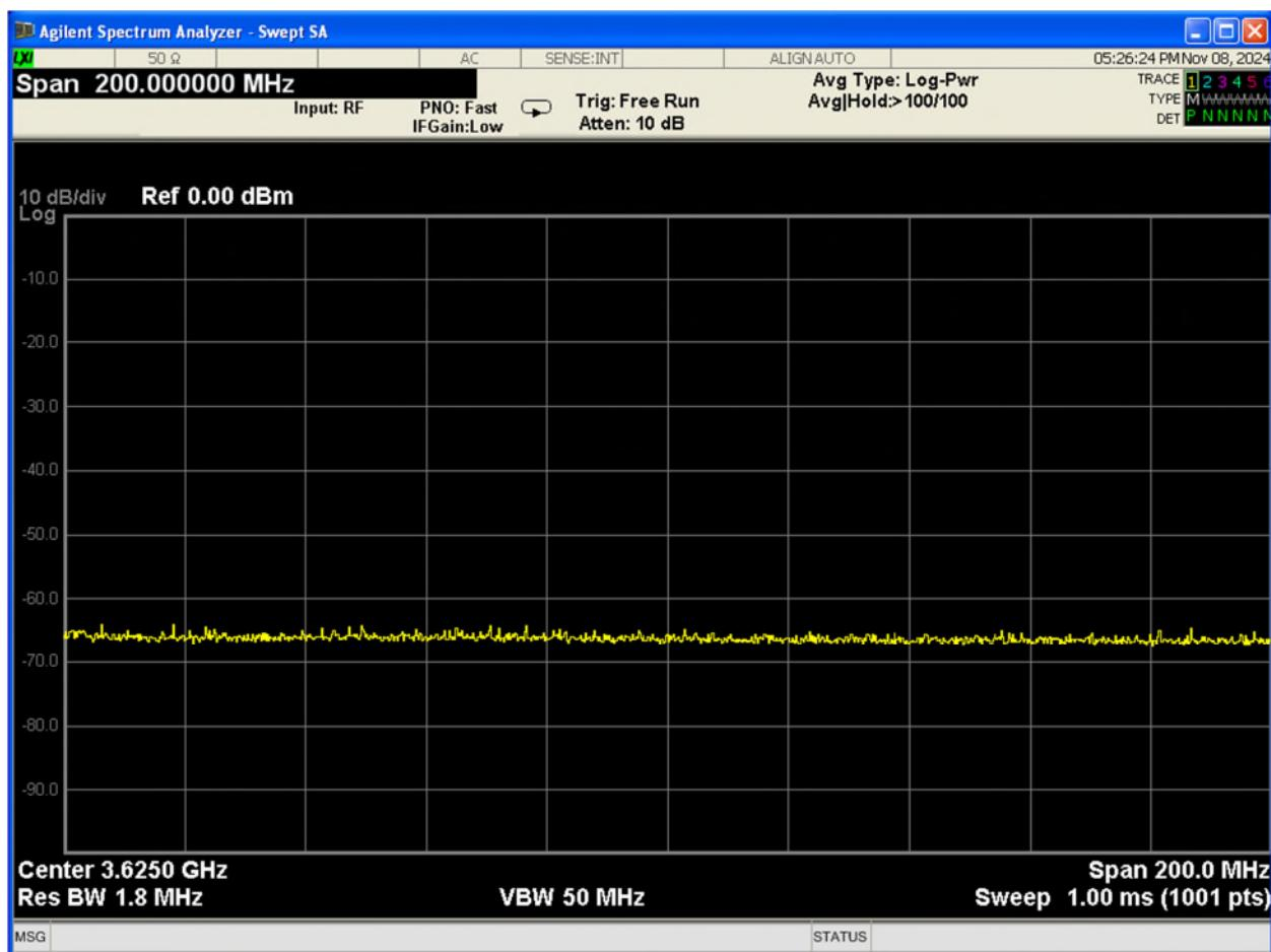
Heartbeat responseCode=501 (SUSPENDED\_GRANT) in First Heartbeat Response was verified via logs. RF transmissions were monitored from start of test and there was no transmission during the test
