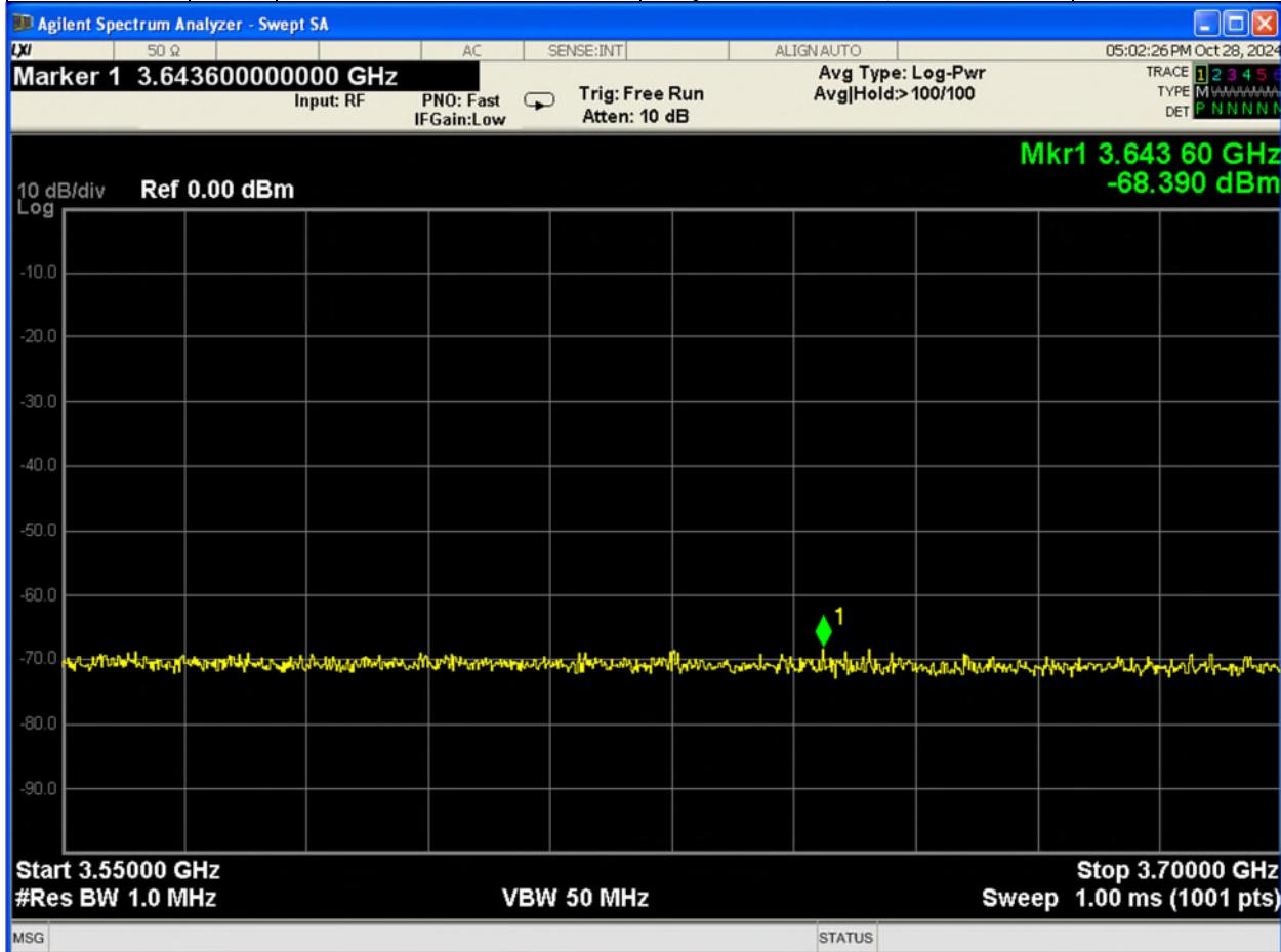
Domain Proxy Unsupported SAS protocol version (responseCode 100) was verified via logs. The EUT did not transmit.
