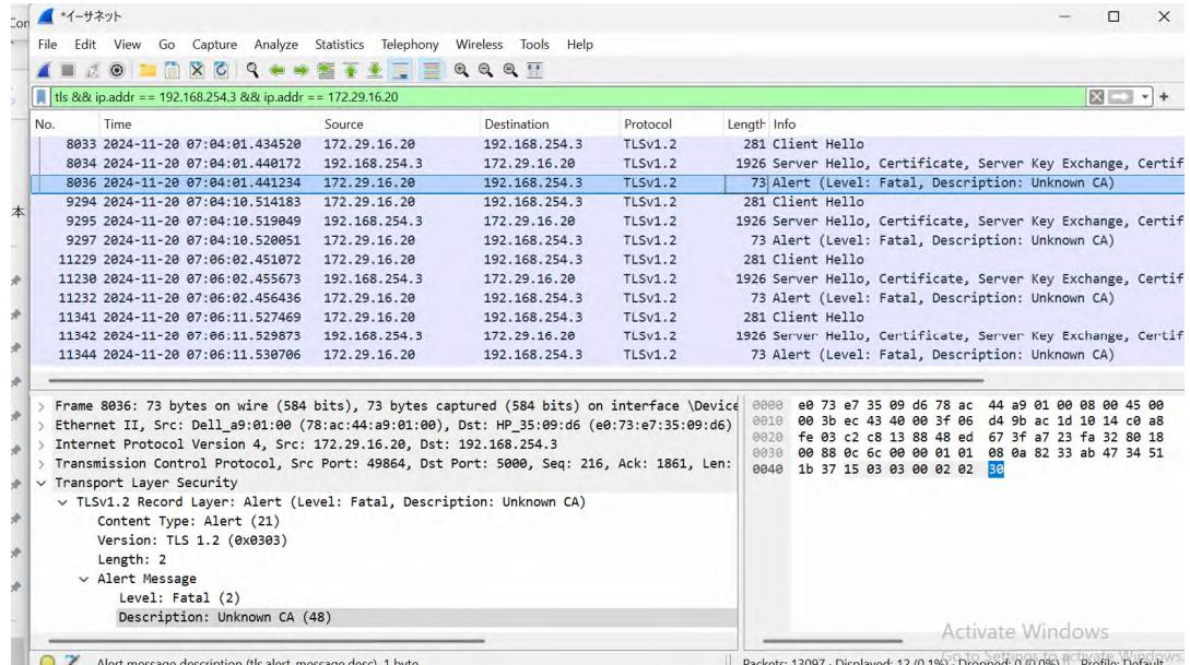
6. Registration request message is not received at Test Harness (authentication fails)
