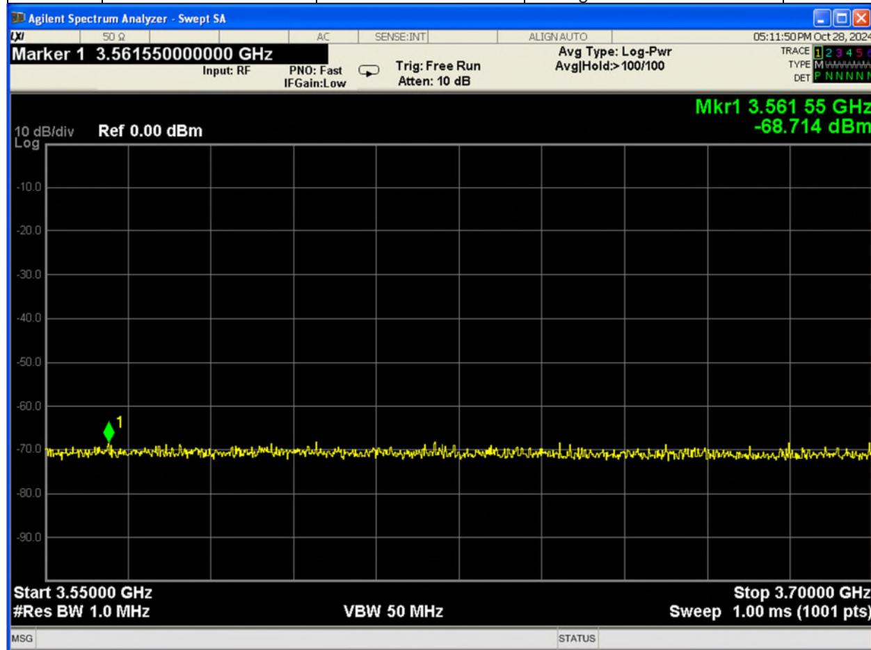
Unsuccessful Grant responseCode=400 (INTERFERENCE) was verified via logs. The EUT was monitored for greater than 60 seconds after REG message sent. No transmissions during test occurred.
