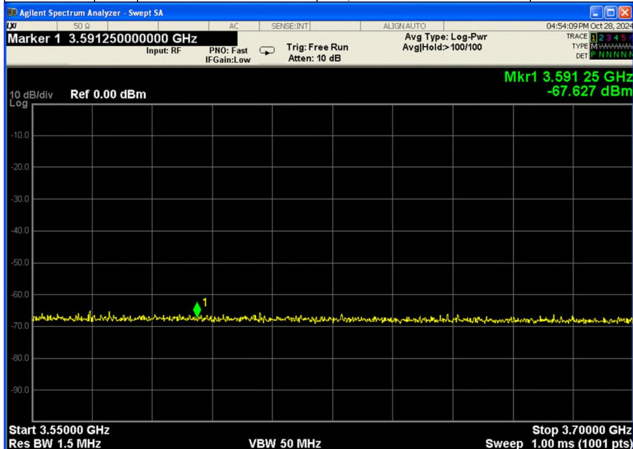
Domain Proxy Pending registration (responseCode 200) was verified by logs. The EUT did not transmit
