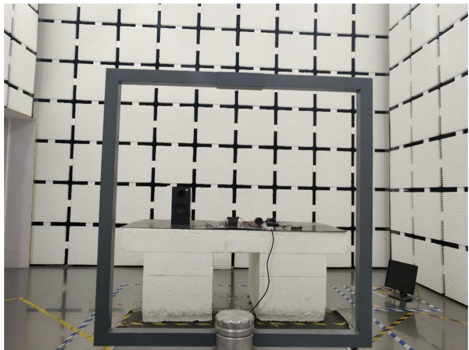
Radiation Emission Test Setup (Below 30MHz)
