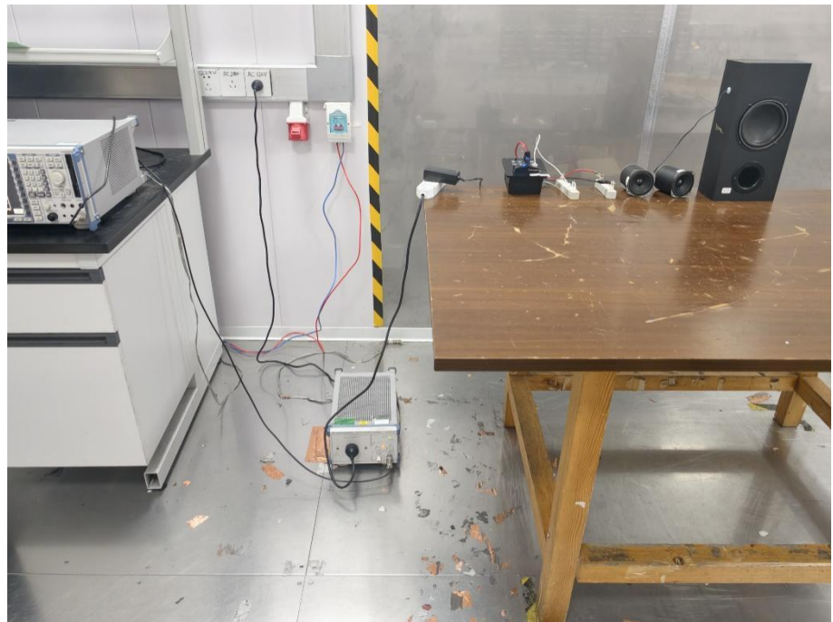
Conducted Emission Test Setup
