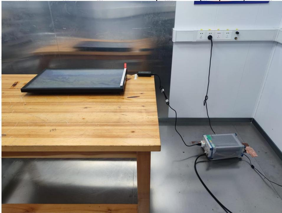
**Emissions in frequency bands (below 1GHz)(Adapter 2)**
