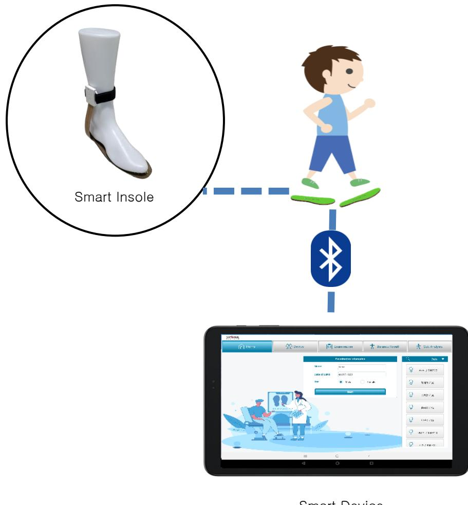
After the user wears the smart insole, the smart insole and smart devices (smartphone, tablet, etc.) are connected via Bluetooth to measure and analyze the user's walking data.
