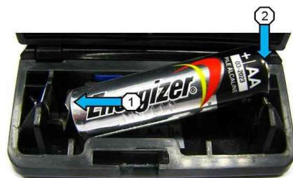
Insert a fresh AA battery as indicated in illustration, be sure to first insert from the negative terminal. Pay special attention to the correct polarity of the battery
