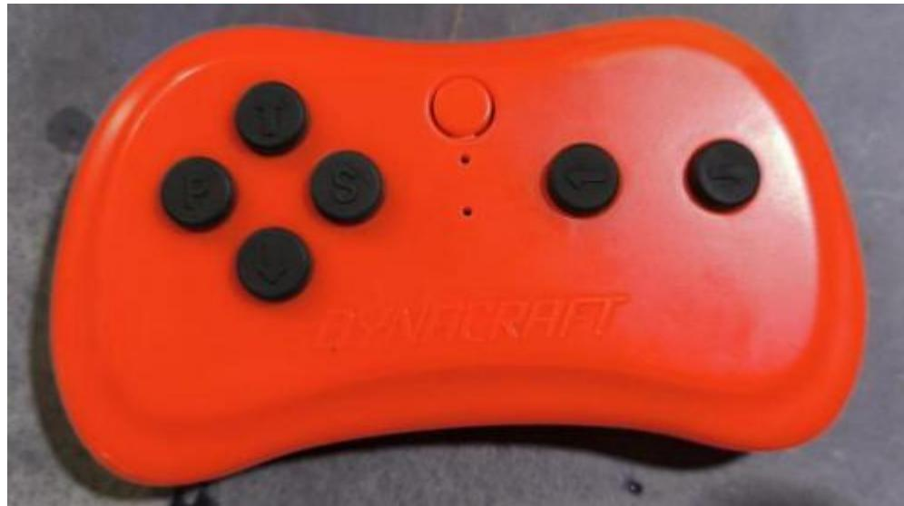
△ : after press, control the car forward, loosen the stop;
