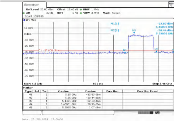
Out Of Band Emission IEEE 802.11ax_Channel 50_160MHz_Antenna 0_RU&Index SU
