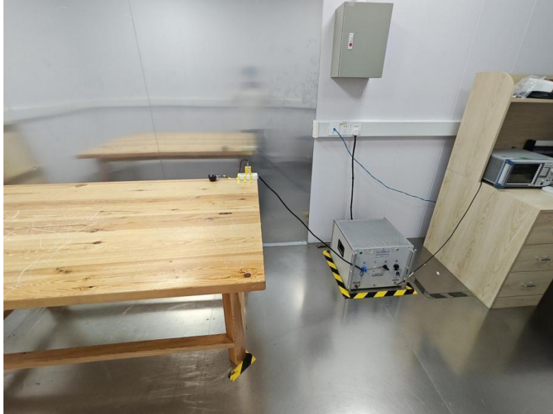
Radiated Emissions From 30M-1GHz
