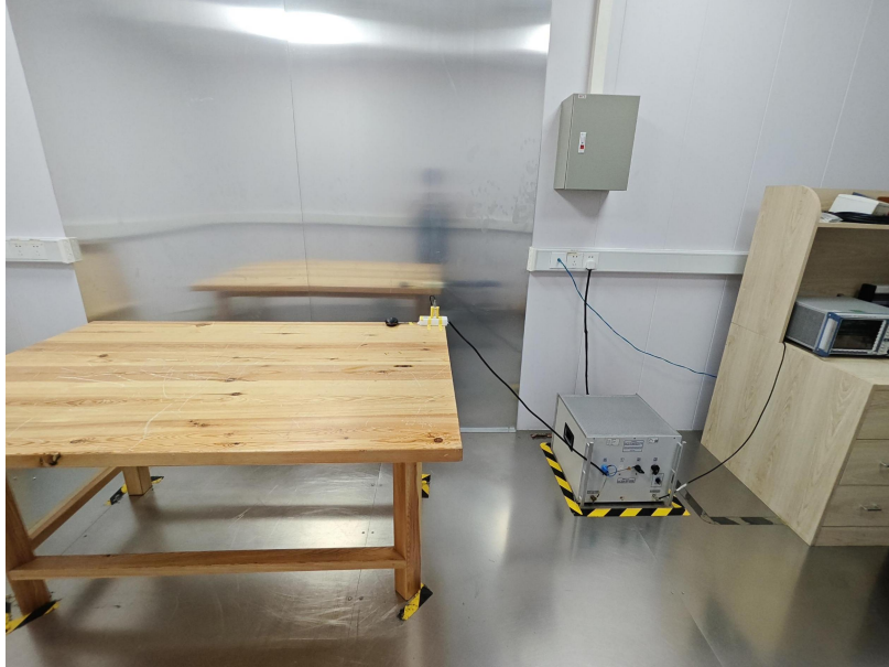
Radiated Emissions From 30M-1GHz
