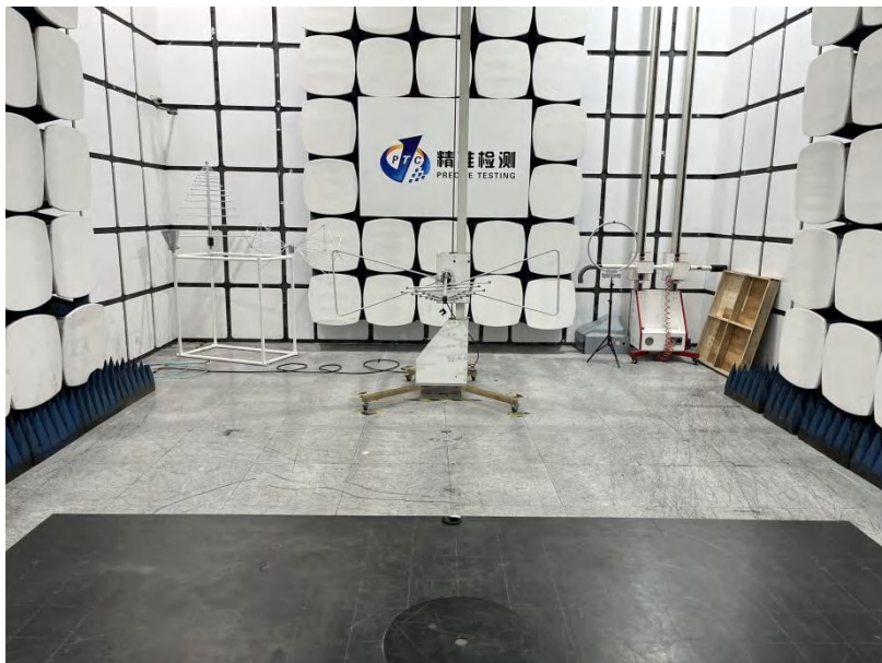
Radiated Emissions From 30M-1GHz
