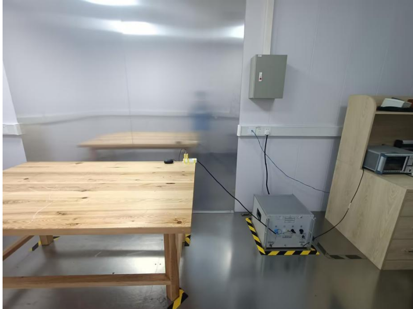
Radiated Emissions From 30M-1GHz
