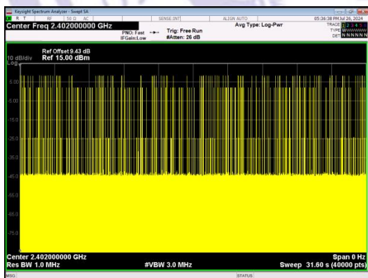
Number of Pulses in 31.6 seconds \pi/4 DQPSK_2-DH5
