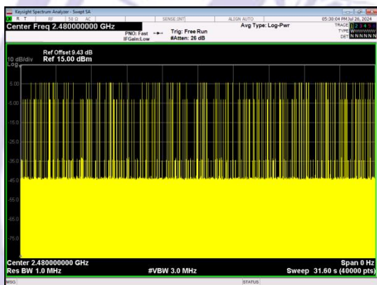
Number of Pulses in 31.6 seconds GFSK_DH5
