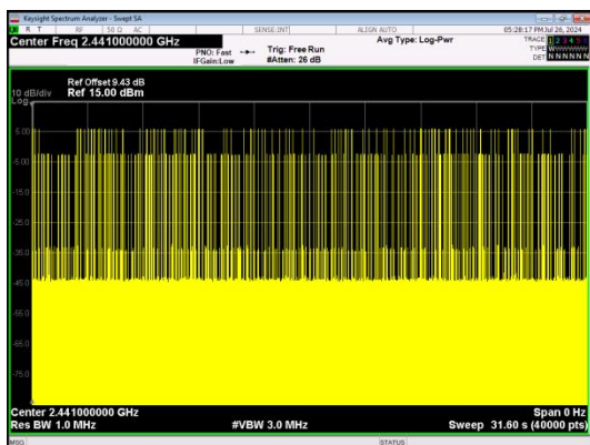
Number of Pulses in 31.6 seconds GFSK_DH5
