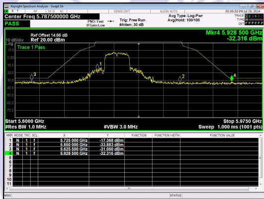
Out Of Band Emission IEEE 802.11n_Channel 151_40MHz_Antenna 0
