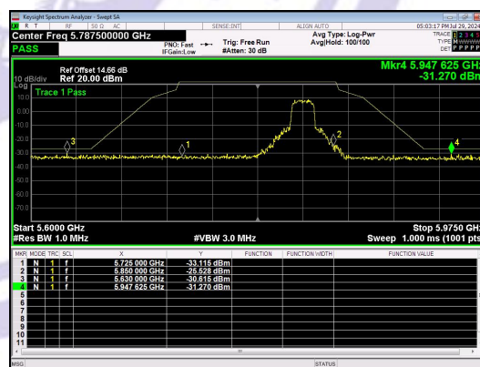
Out Of Band Emission IEEE 802.11n_Channel 165_20MHz_Antenna 0
