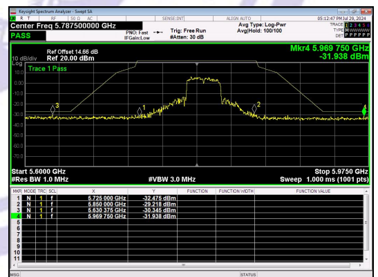
Out Of Band Emission IEEE 802.11n_Channel 159_40MHz_Antenna 0
