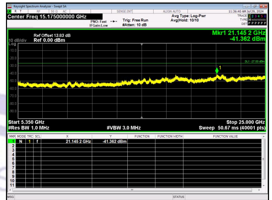
Spurious Emission:5350~25000.0 MHz IEEE 802.11n_Channel 48_20MHz_Antenna 0
