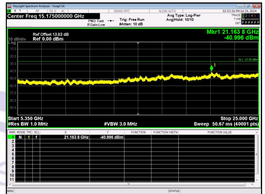
Spurious Emission:15.175~25.000 GHz IEEE 802.11n_Channel 46_40MHz_Antenna 0
