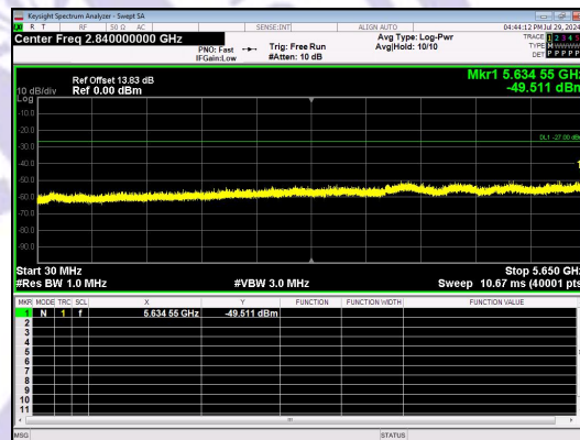
Spurious Emission:30.0~5650 MHz IEEE 802.11n_Channel 157_20MHz_Antenna 0
