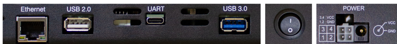
Figure 2-3 I/O interfaces for SIRIUS
