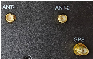
Figure 2-2 Antenna ports for SIRIUS
