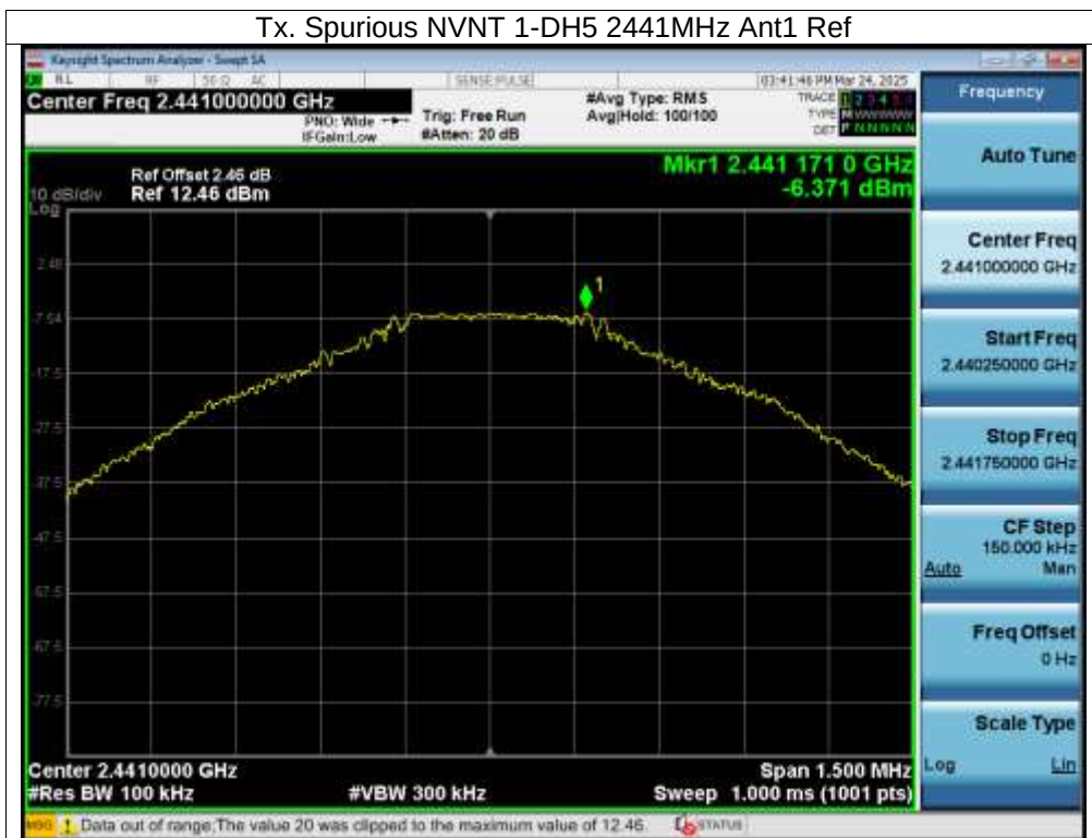
Tx. Spurious NVNT 1-DH5 2441MHz Ant1 Emission
