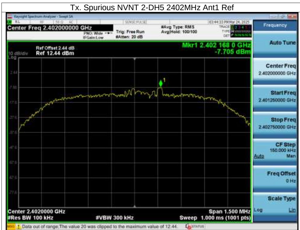
Tx. Spurious NVNT 2-DH5 2402MHz Ant1 Emission
