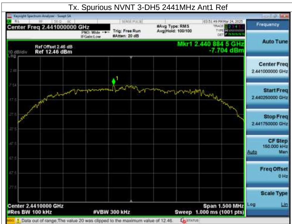
Tx. Spurious NVNT 3-DH5 2441MHz Ant1 Emission
