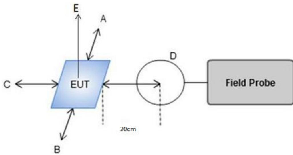
Note: Position A: Front of EUT; Position B: Left of EUT; Position C: back of EUT; Position D: Right of EUT; Position E: Top of EUT(20 cm measure distance)
