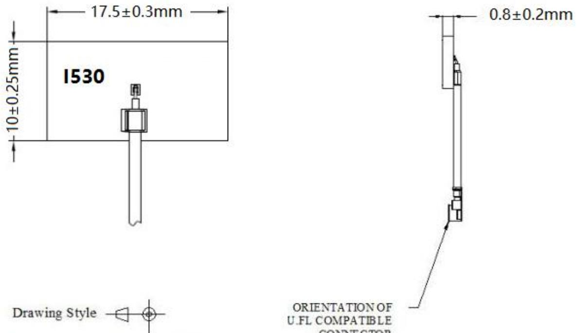
Tape's tolerances are all in  $\pm 0.5\text{mm}$
