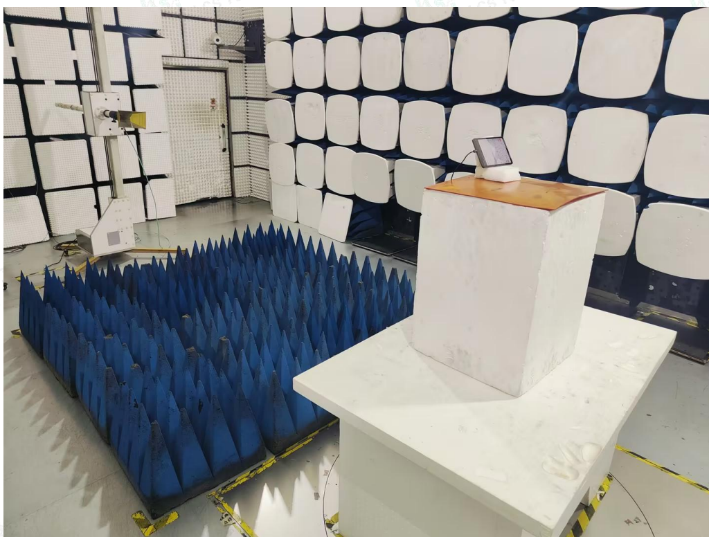
Radiated Emissions Measurement (Above 1GHz)
