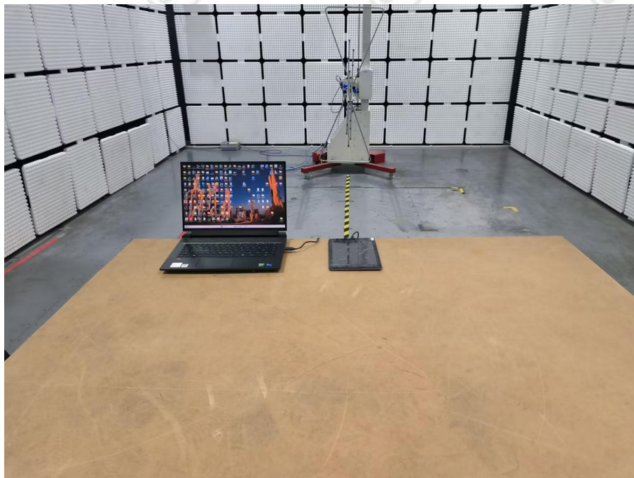
Radiated spurious emission Test Setup-1(Below 1GHz)
