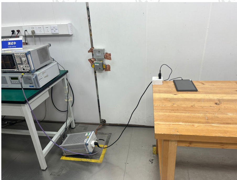
Conducted Emissions Test Setup
