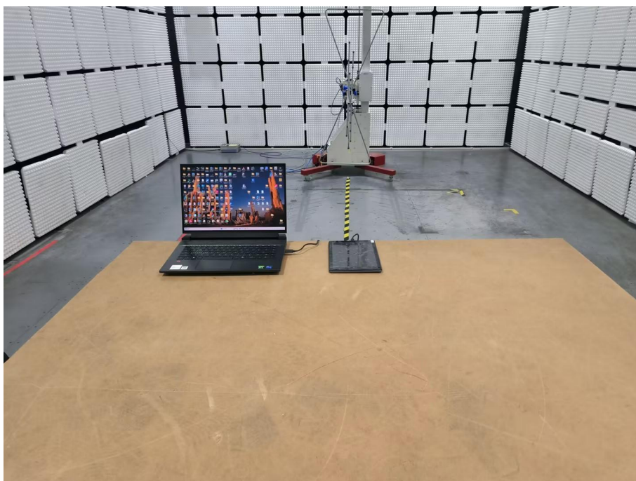
Radiated spurious emission Test Setup-1(Below 1GHz)
