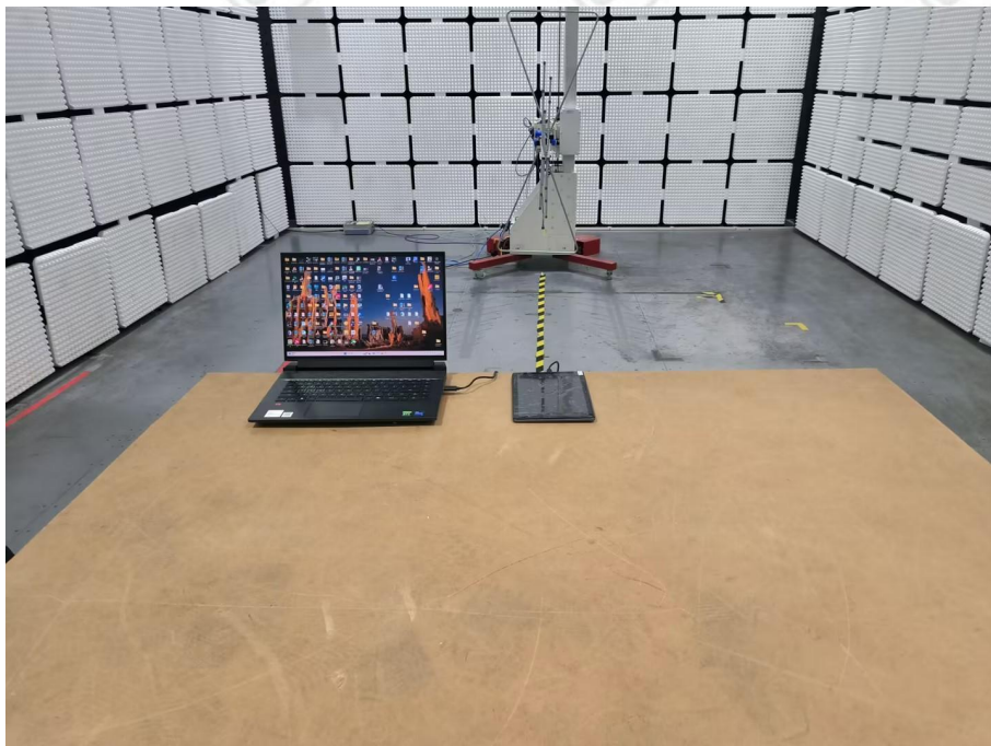
Radiated spurious emission Test Setup-1(Below 1GHz)
