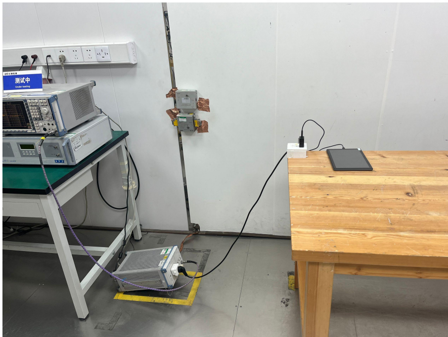
Conducted Emissions Test Setup
